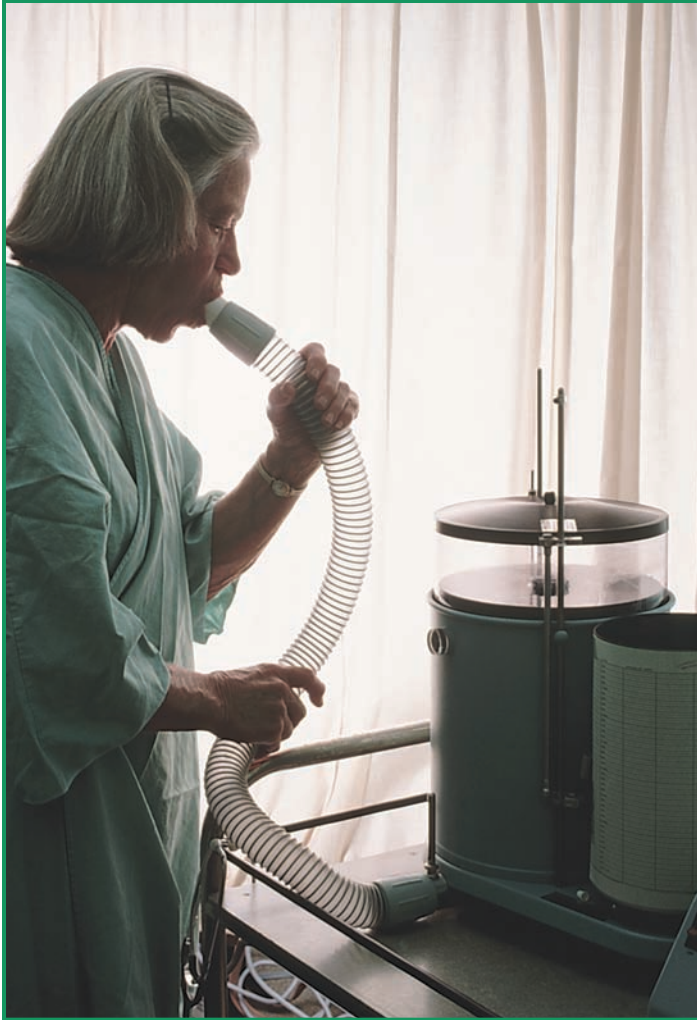
Figure 6.4 The woman in this picture is using a spirometer, which allows respiratory physiologists to determine the major respiratory volumes for an individual and to assess his or her respiratory function.
