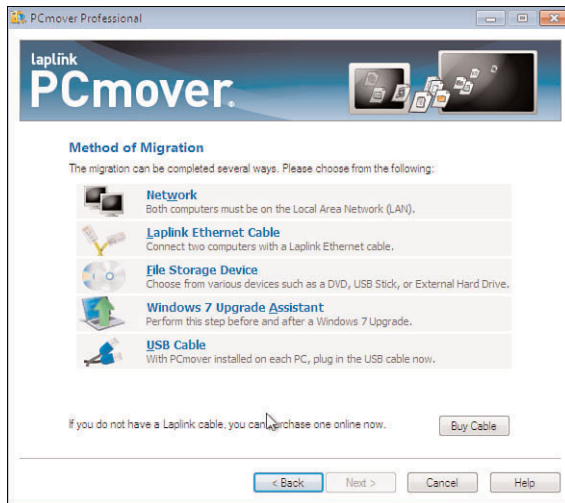
FIGURE 5.19 Choose the right kind of transfer method; unless there's a really good reason to use USB, we highly recommend transferring via a network connection.
