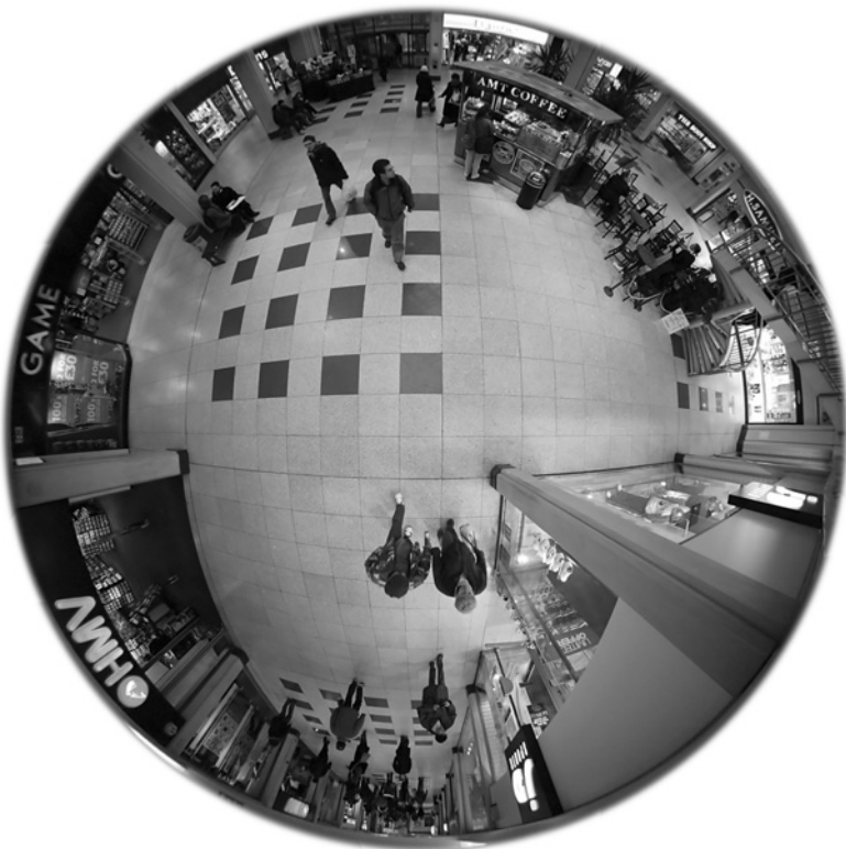
Figure 6.18b Panoramic view produced by the lens when the camera is ceiling mounted
