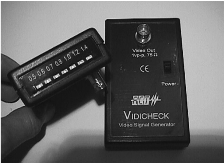
Figure 2.31 A typical hand-held test instrument for testing co-axial cables, checking video signal levels, verifying camera output, etc. (Courtesy of ACT Meters Ltd)
