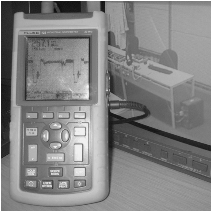
Figure 13.3 A hand-held oscilloscope is far more suited to CCTV testing than a full-sized bench model. Units such as this incorporate rechargeable batteries, and have default settings to enable rapid display of analogue video waveforms
