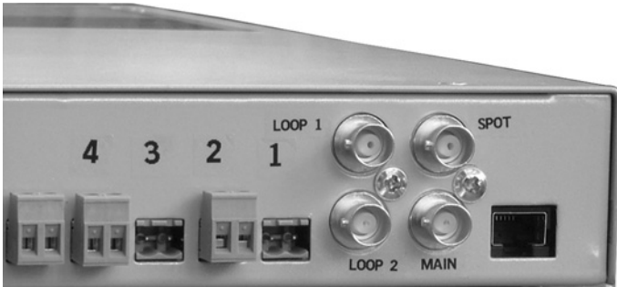
Figure 2.18 A DVR/MUX which offers direct twisted pair video signal input. (Photo courtesy of Tecton Ltd)
