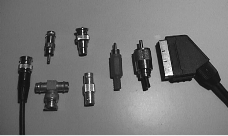
Figure 2.29 Range of connectors. From left to right: BNC crimp, BNC T coupler, BNC straight coupler, two variations of BNC/phono adapter (top), Phono, UHF, SCART.
