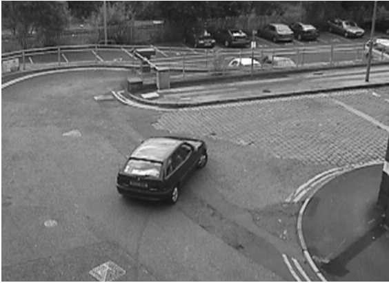
Figure 5.18 The only significant movement in this clip is that of the vehicle, and therefore the majority of the video information only needs to be transmitted for the first frame
