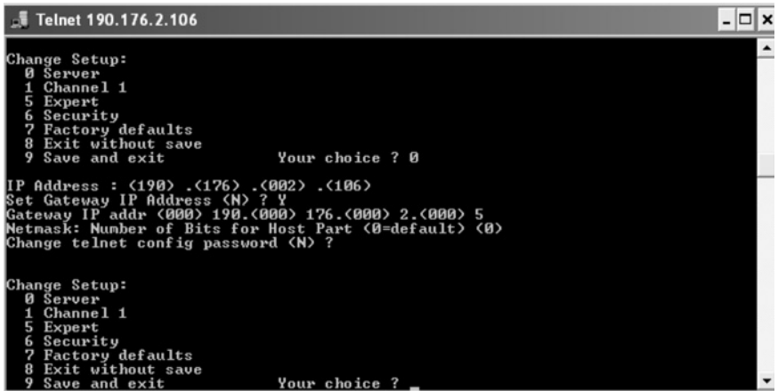
Figure 11.11c Typical Telnet software utility used to set up a remote network device such as an IP camera, once an IP address has been assigned using ARP
