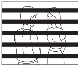
Odd field (312.5 lines PAL) (262.5 lines NTSC)
