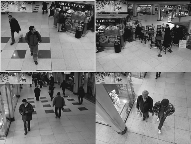
Figure 6.18c Typical example of the video output available from this camera. Four corrected images in quad display created from the original panoramic image. It would be easy to believe that there are four separate cameras in the installation (Photos and images courtesy of Vista)
