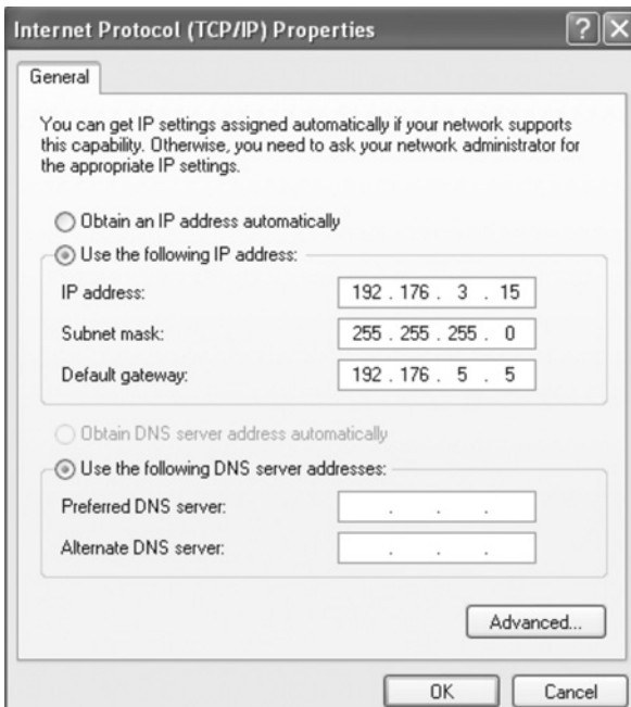
Figure 11.11a TCP/IP set-up screen from Microsoft Windows XP, used to set up a static IP address on the PC itself
