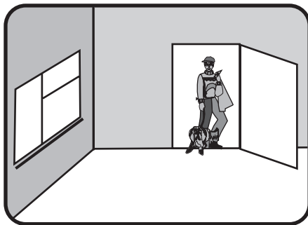
Figure 6.14b During the daytime the iris closes down in proportion to the light level around the doorway, resulting in the person having a silhouette appearance
