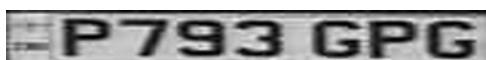
Figure 6.20c Vehicle number plate, digitally derived from the images from the IR camera. (Photos courtesy of Vista)
