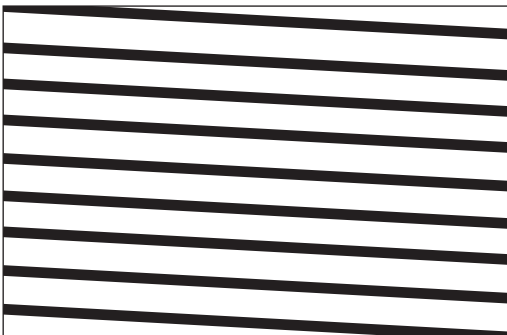
Figure 7.7 Effects of maladjusted timebase controls
