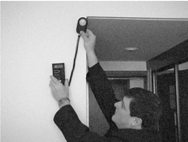
Figure 3.12 When using a light level meter, take the reading at the camera location
