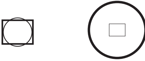
(a) A 1/3" format lens fitted to a 2/3" format camera
