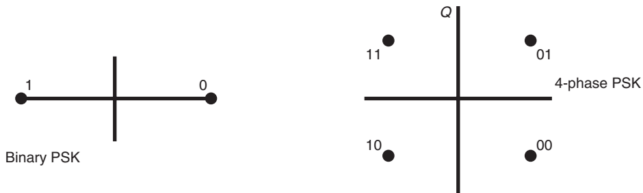
Figure 3.15 Phasor constellations for BPSK and QPSK.
