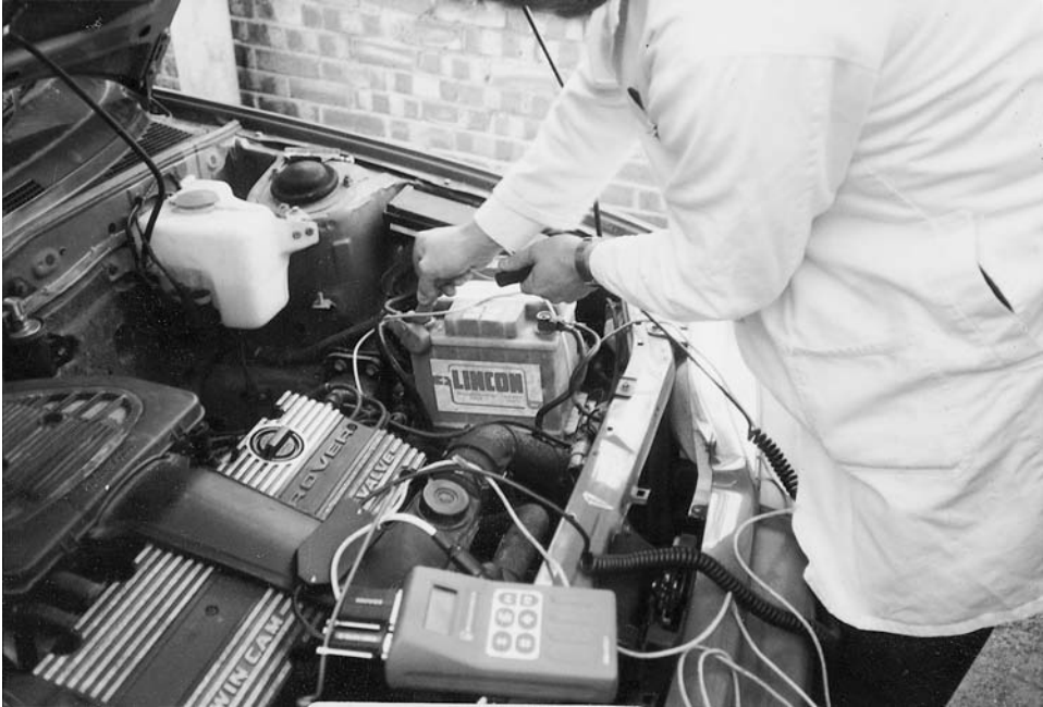
Fig. 3.14 Connecting to the power supply
