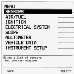
Fig. 4.13(b) An overview of available test functions from the MENU key of the Bosch PMS 100 portable oscilloscope
