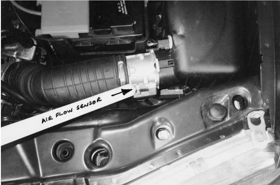
Fig. 5.40 A 'hot-wire' air flow sensor
