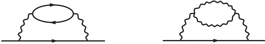
Figure 7.2. The first diagram shows a typical contribution to the self-energy of the electron. The virtual particle/anti-particle pair behaves as a small electric dipole, thereby screening the electron charge. Turning to quarks and the strong interaction, in quantum chromodynamics the diagrams of the first kind (where now the wavy line denotes a gluon, rather than a photon) are accompanied by additional ones of the second kind, since the gluons are themselves charged. A direct calculation shows that the anti-screening effect wins, leading to asymptotic freedom .
