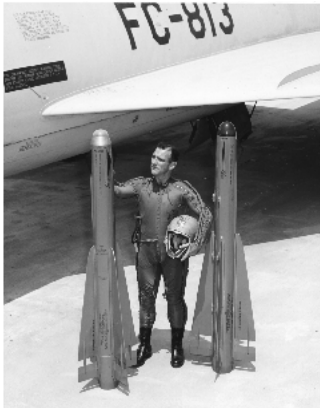
Figure 9.1. GAR-2A infrared Guided Aircraft Rocket (left) developed by US Air Force, beside James J O'Reilly, engineering test pilot for the Hughes Aircraft Company. In production from 1956, some 16 000 of the original design were produced. Reproduced with permission of HRL Laboratories, Malibu, CA.
