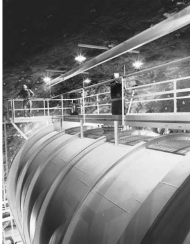
Figure 10.8. The chlorine detector of Davis for the detection of solar neutrinos in the about 1400 m deep Homestake Mine in Lead, South Dakota (USA) in about 1967. The 380 000 l tank full of perchloro-ethylene is shown. Dr Davis is standing above. (Photograph from Brookhaven National Laboratory.)
