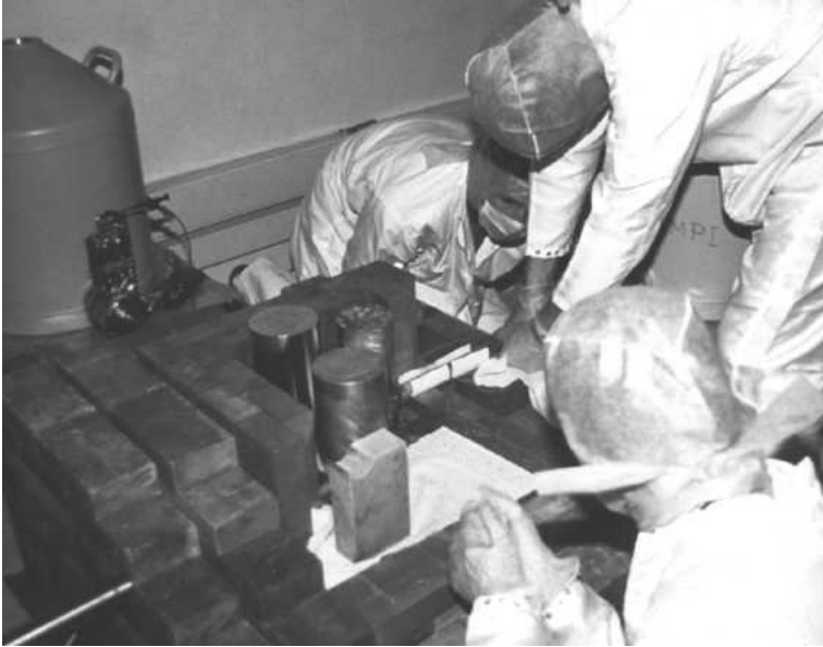
Figure 7.10. Photograph of the installation of enriched detectors in the Heidelberg–Moscow experiment (with kind permission of H V Klapdor-Kleingrothaus).
