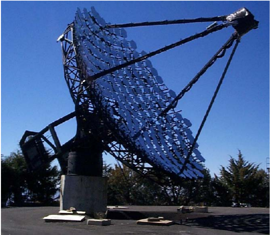
Figure 1.3. The Whipple 10 m gamma-ray telescope. Note the ‘10 m’ refers only to the aperture of the optical reflector; the effective collection area is >5 \times 10\,000\text{ m}^2 so that the gamma-ray ‘aperture’ is 120 m.
