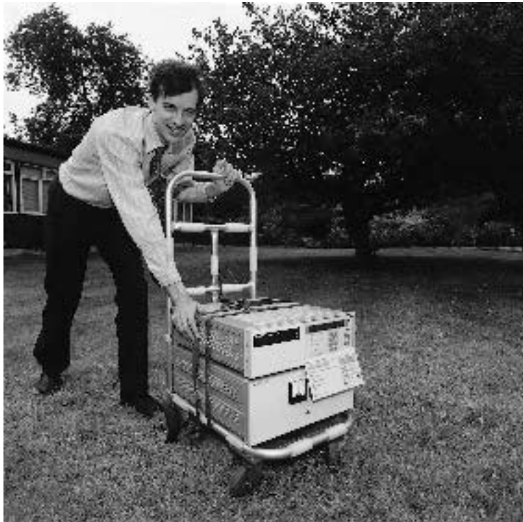
Figure 7.1. John Davis, of NPL, prepares an atomic clock for a flight between London and Washington in a demonstration of Einstein's relativity for the BBC Horizon television programme.
