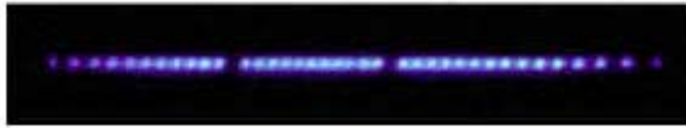
Figure 8.5. A string of mercury ions is held in a trap at the National Institute for Standards and Technology. Such ions can be used as frequency standards by exposing them to microwave radiation at the hyperfine transition frequency.
