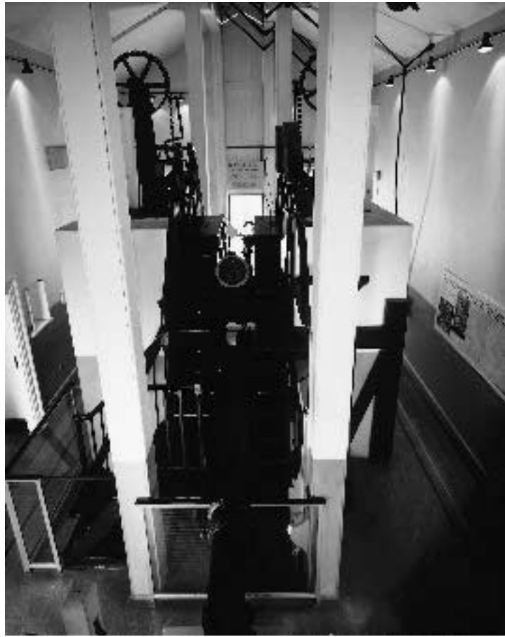
Figure 5.1. Until the late twentieth century all our timekeeping was based on the timing of stars as they crossed the meridian. This specialised telescope, the Airy Transit Circle, kept time at the Royal Observatory in Greenwich from 1851 to 1927, when it was replaced with more modern instruments. The object lens of the telescope is the grey circle in the centre of the picture. In 1884 the location of the telescope was internationally agreed to define the prime meridian of longitude.
