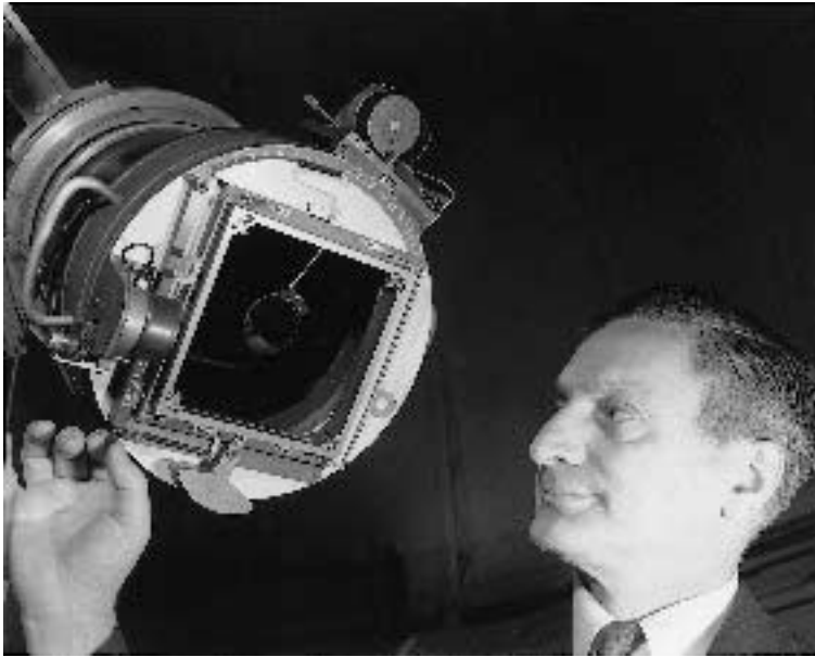
Figure 3.2. William Markowitz, of the US Naval Observatory, with the Moon camera he designed for the measurement of Ephemeris Time. In this picture the back of the camera has been removed to reveal the circular filter which slowly tilts to prevent the image of the Moon drifting against the stars.
