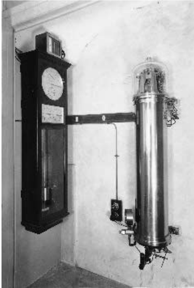
Figure 2.3. The Shortt free pendulum clock was the mainstay of astronomical timekeeping in the 1920s and 1930s. The vacuum chamber on the right contains the freely swinging “master” pendulum which transmits electrical signals to the “slave” pendulum in the cabinet on the left. This one operated at NPL from 1927 to 1959.
