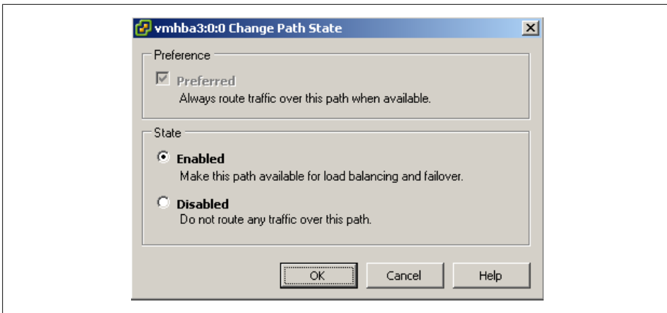
Figure 2-17. Enabling or disabling a path
