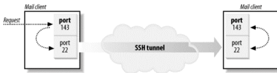
Figure 3-1. IMAP over SSH tunnel
