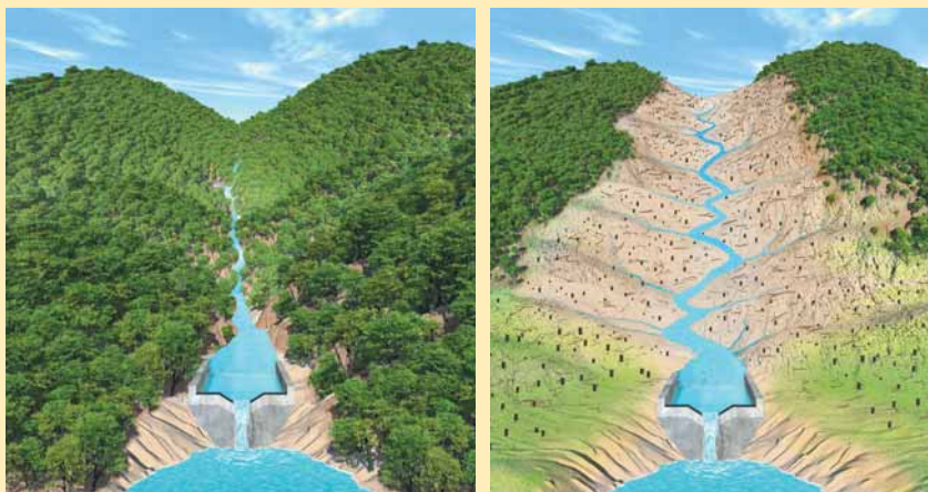
Figure 2-1 Controlled field experiment to measure the effects of deforestation on the loss of water and soil nutrients from a forest. V-notched dams were built into the impenetrable bedrock at the bottoms of several forested valleys (left) so that all water and nutrients flowing from each valley could be collected and measured for volume and mineral content. Baseline data were collected on the forested valley (left) that acted as the control site. Then all the trees in one valley (the experimental site) were cut (right) and the flows of water and soil nutrients from this experimental valley were measured for three years.
