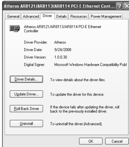
Figure 20-2: The device Properties dialog box shows the driver version number and release date.
