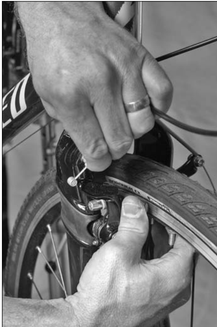
Figure 8-6: Undoing the quick- release.
