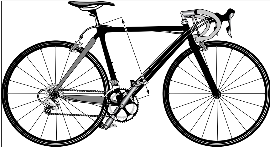
Figure 19-3: How frame size is measured.
