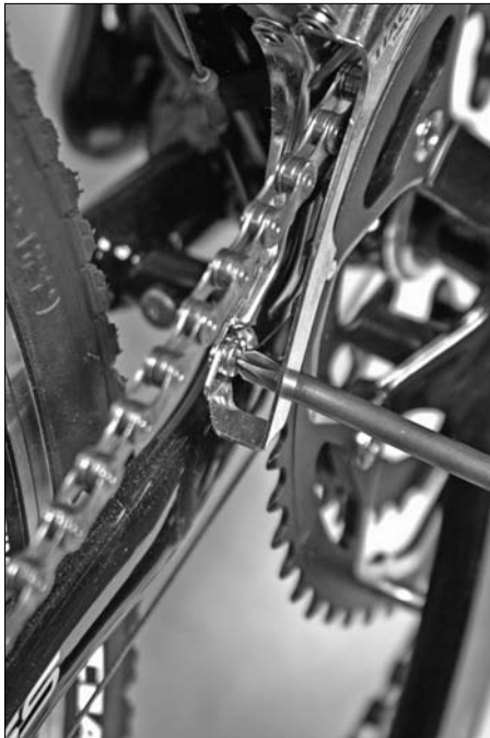
Figure 14-13: Pulling the cage apart.
