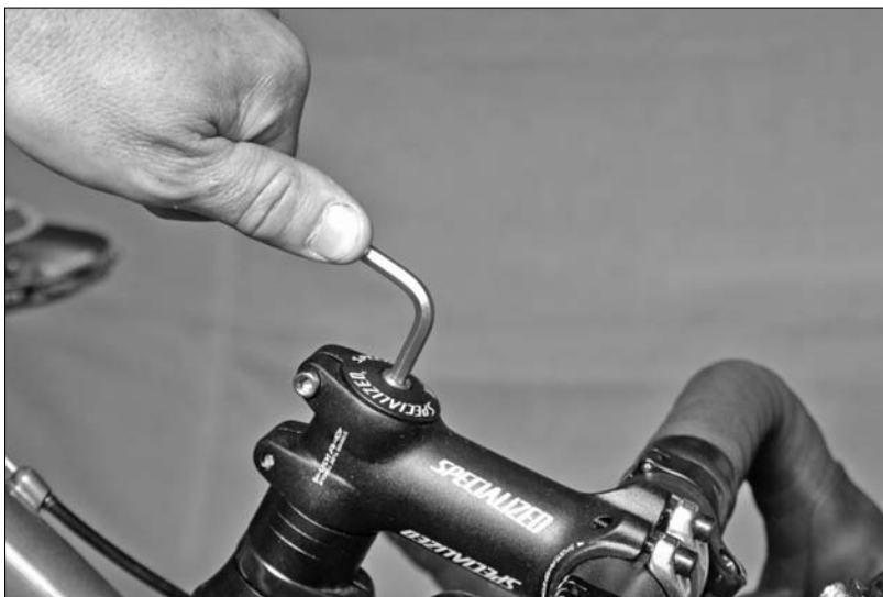
Figure 15-11: Loosening the top cap.
