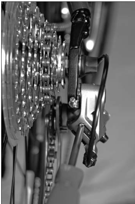
Figure 14-6: Adjusting the H screw.
