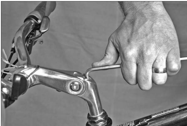
Figure 15-18: Loosening the socket head bolt.
