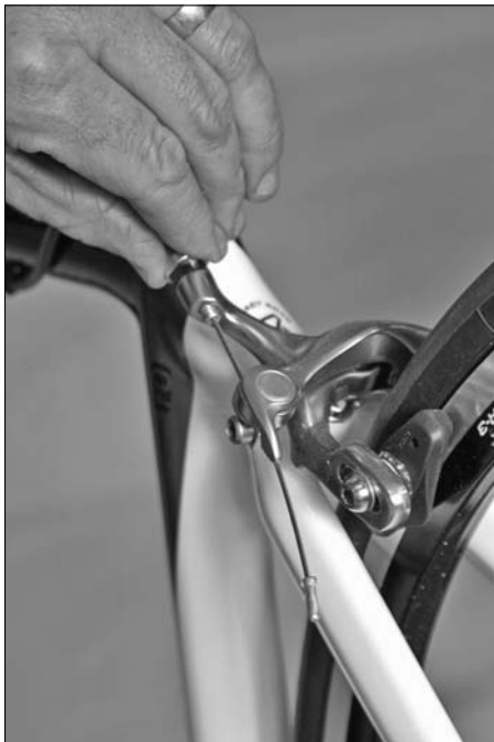
Figure 8-16: Adjusting the cable on center- mount brakes.
