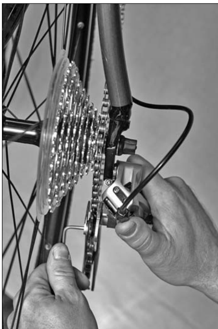
Figure 14-3: Loosening the top jockey wheel.
