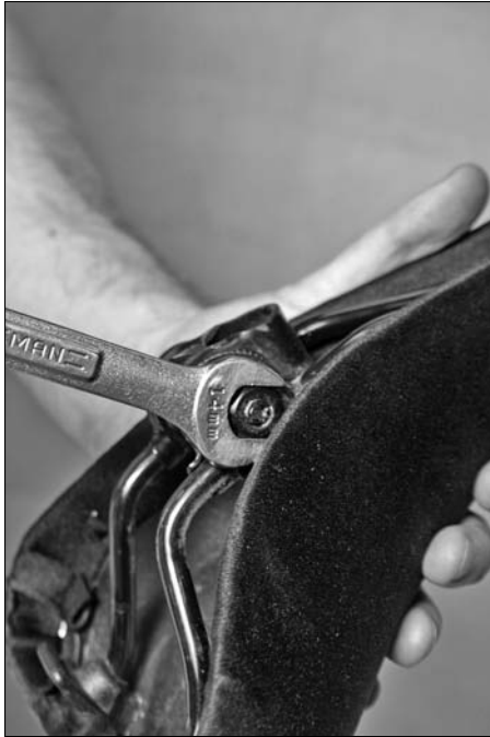
Figure 9-4: A traditional saddle clamp.
