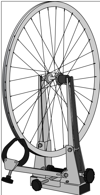
Figure 7-12: Using a truing stand
