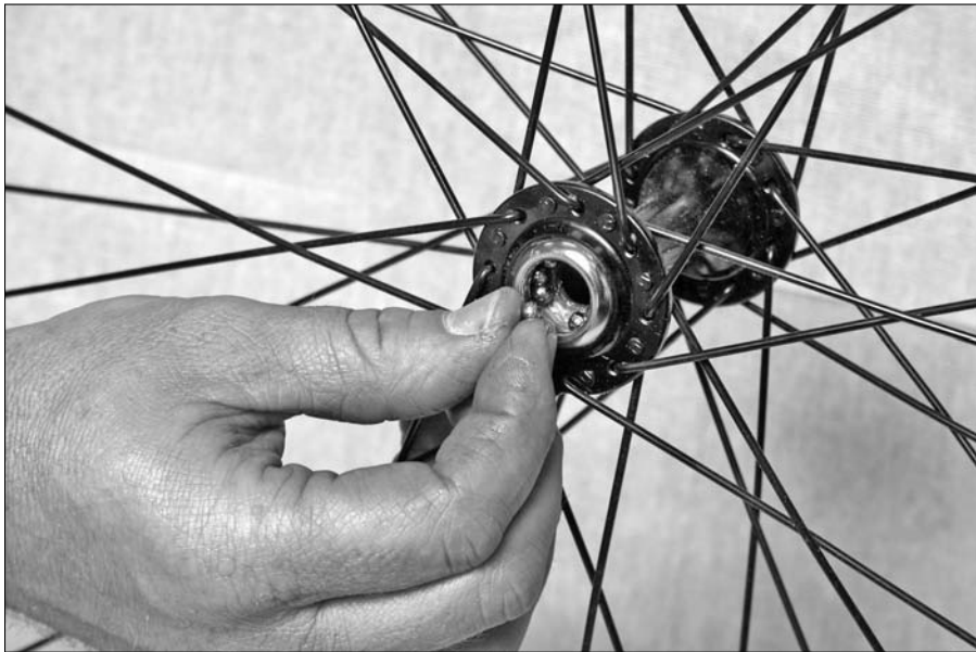
Figure 7-7: Removing the bear- ings.
