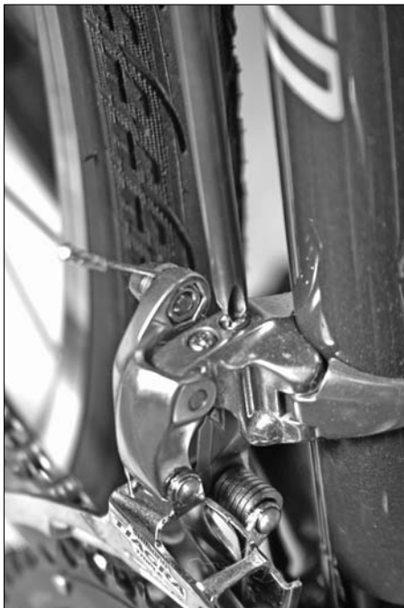
Figure 14-14: Adjusting the L-limit screw.
