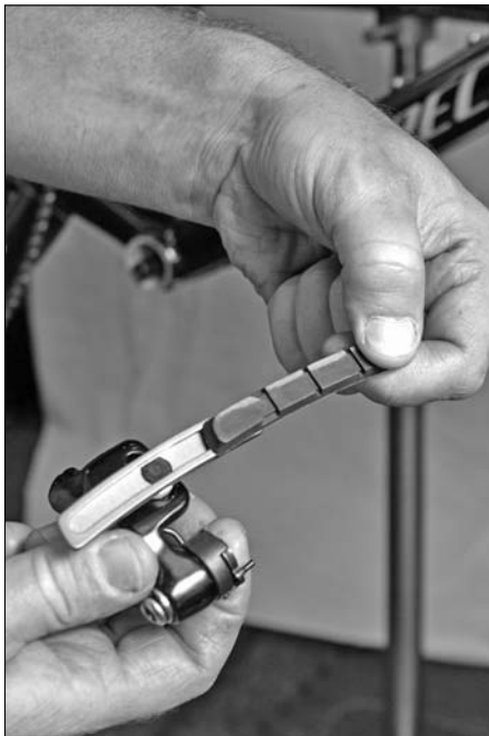
Figure 8-10: Removing the brake pad.
