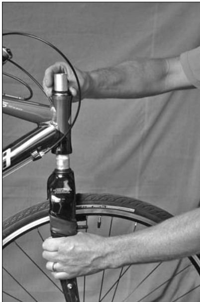
Figure 15-15: Removing the fork.
