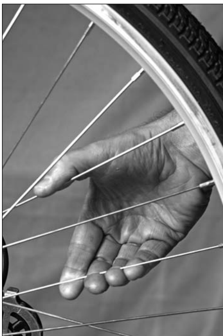
Figure 7-13: Feeling for loose areas.
