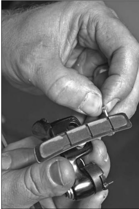
Figure 8-9: Removing the brake- pad pin.
