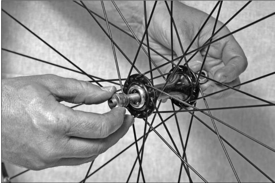
Figure 7-6: Removing the axle.
