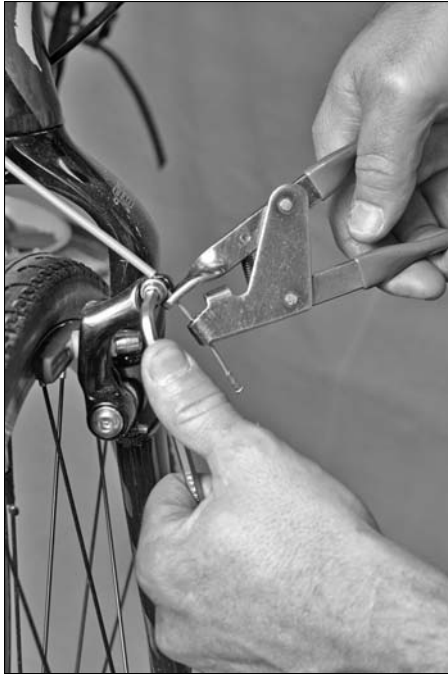
Figure 8-11: Using a fourth-hand tool.
