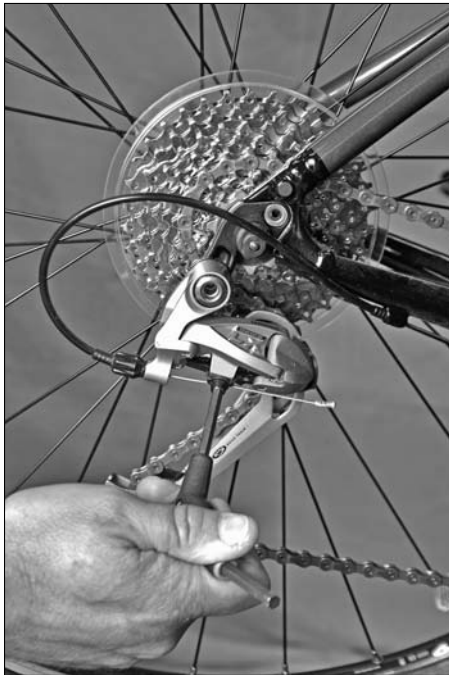
Figure 14-8: Attaching the cable.
