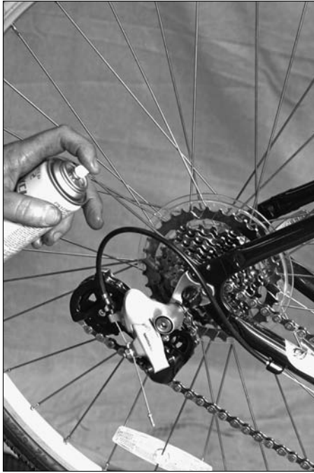
Figure 16-2: Degreasing various parts of a bike.
