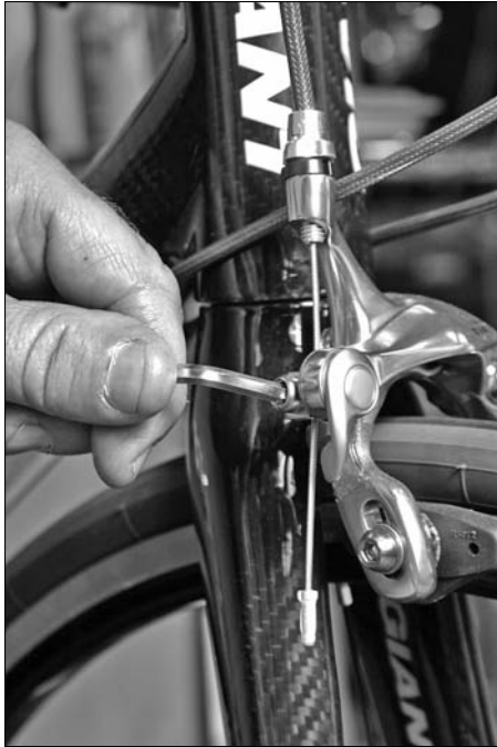
Figure 8-15: Adjusting center- mount brakes.
