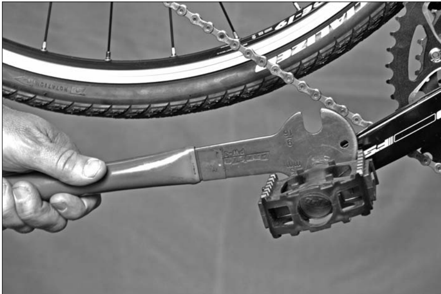
Figure 13-1: Using a pedal wrench to remove a pedal.
