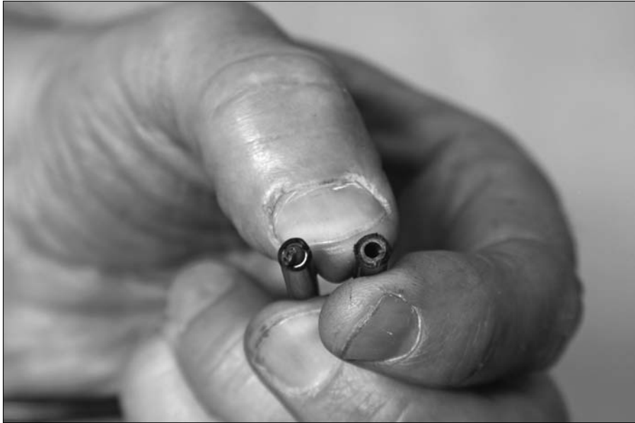
Figure 8-22: Properly cut cable housing.
