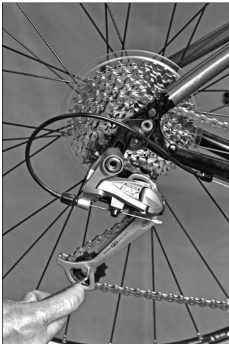
Figure 14-2: Loosening the bottom jockey wheel.
