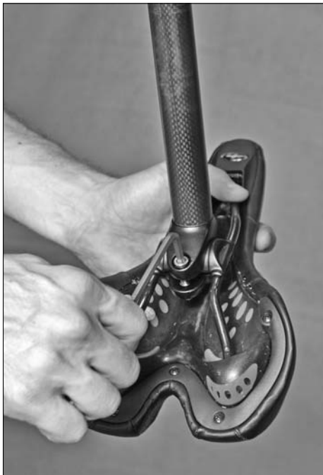
Figure 9-5: One piece saddle clamp.
