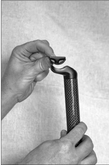
Figure 9-6: One piece saddle dis- assembled.
