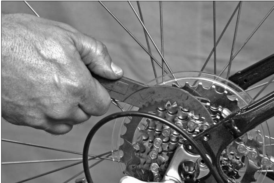
Figure 16-3: Digging out dirt between the cogs.
