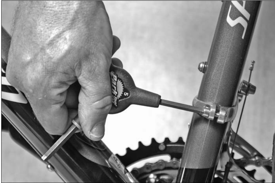
Figure 14-12: Removing the pivot bolt.
