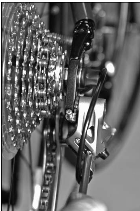
Figure 14-7: Adjusting the L screw.
