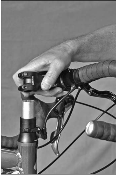
Figure 15-13: Removing the stem.
