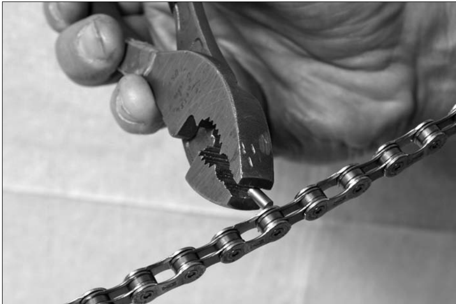
Figure 10-15: Snapping off the replacement pin's head.
