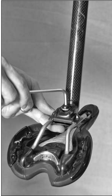
Figure 9-7: Attaching a two-piece clamp.
