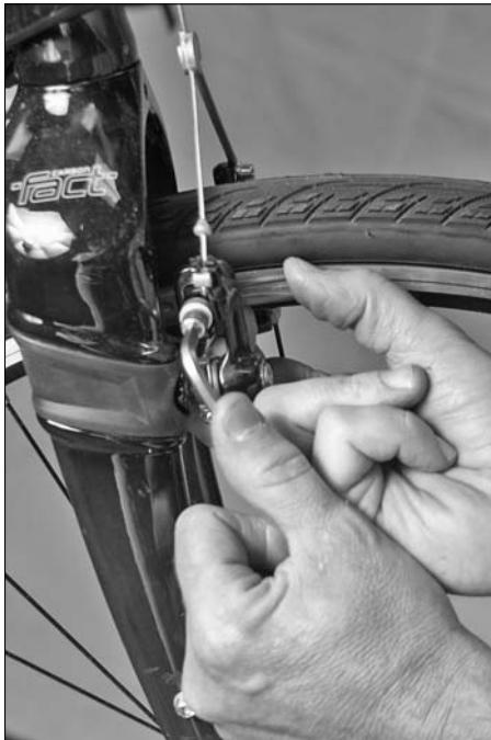
Figure 8-12: Adjusting the brake.
