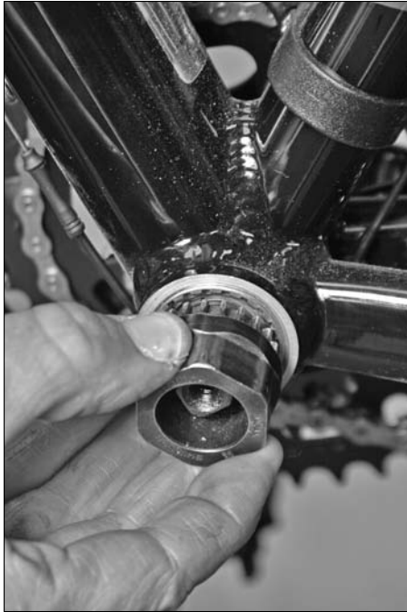
Figure 13-11: Attaching a bottom bracket tool.
