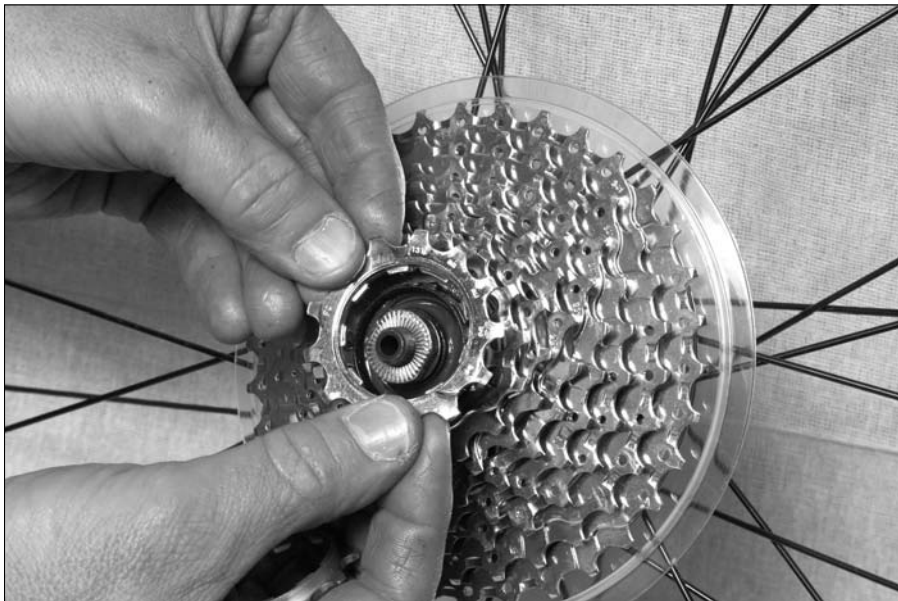
Figure 11-5: Removing the cogs on a cassette
