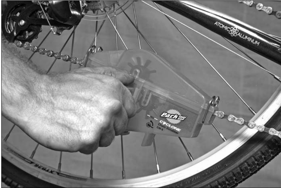
Figure 10-10: A chain cleaning tool takes your cleaning to the next level.
