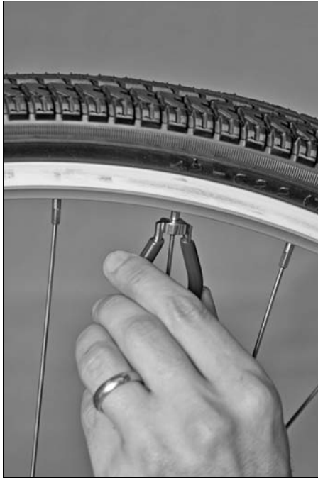
Figure 7-14: Using a spoke wrench.
