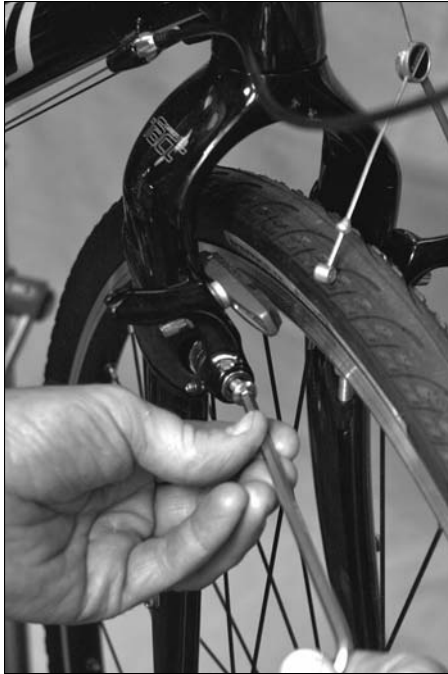
Figure 8-7: Loosening the brake.
