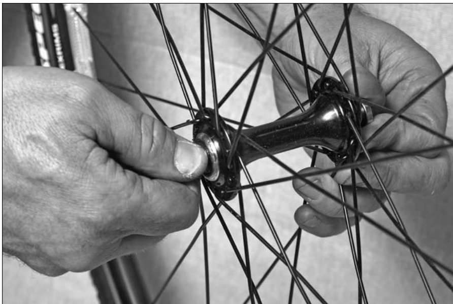
Figure 7-10: Attaching the locknut.
