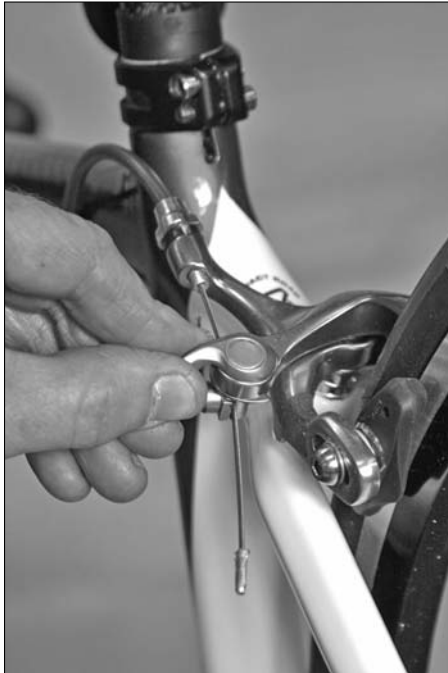
Figure 8-14: Moving the lever on center- mount brakes
