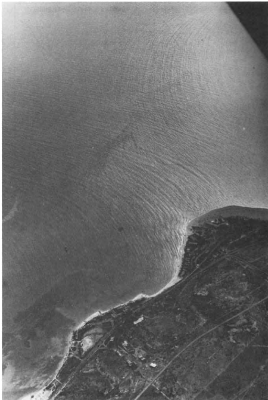
Fig.4. Aerial photograph of the cross-pattern of refracted waves near Manshebu.
