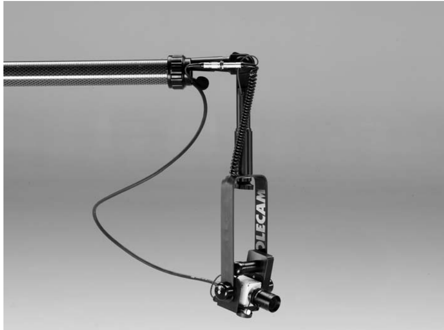
FIG1.24 Polecam head. “Down at the business end, the Toshiba camera sits in the camera head with all controls accessed back with the operator.”
