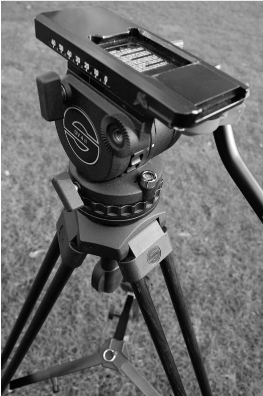
FIG 1.9 SONY Z1 tripod Sachtler 14P. "This Sachtler 14p head and legs is designed for smaller semi-pro cameras but allow you to do smooth pans and tilts as well, unlike many photographic tripods."
