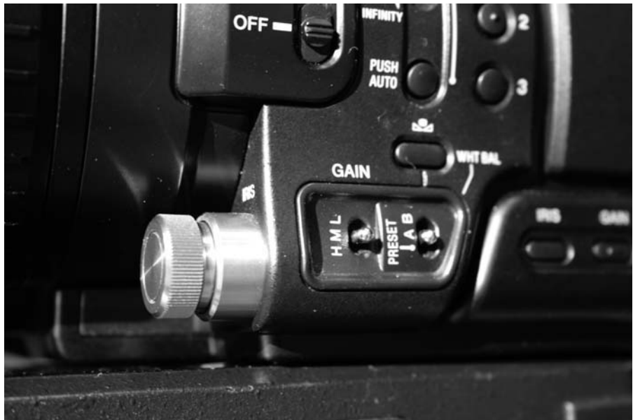
FIG 1.4 SONY Z1 aperture wheel close-up. "Someone at SONY decided to put the aperture ring down here... why I wonder?"
