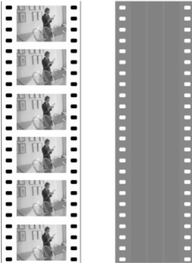
Figure A2.3 In traditional film technique, sound is recorded on magnetic film with the same dimensions as the image allowing simple mechanical synchronization.
