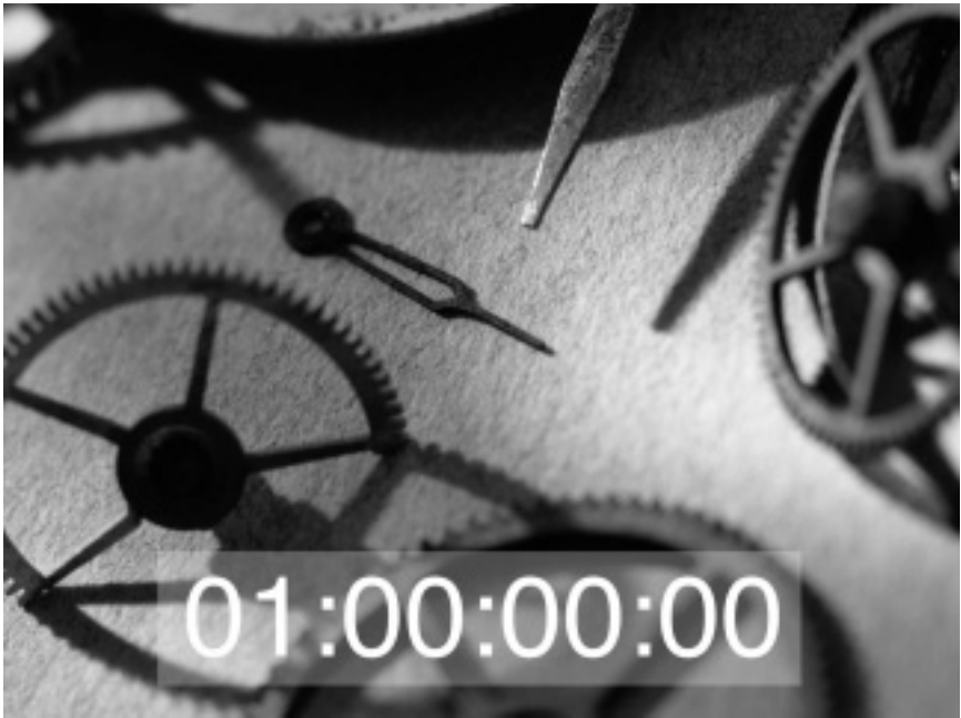
Figure A2.5 In-picture timecode display created by a VITC reader and character inserter. Burnt-in timecode looks similar.
