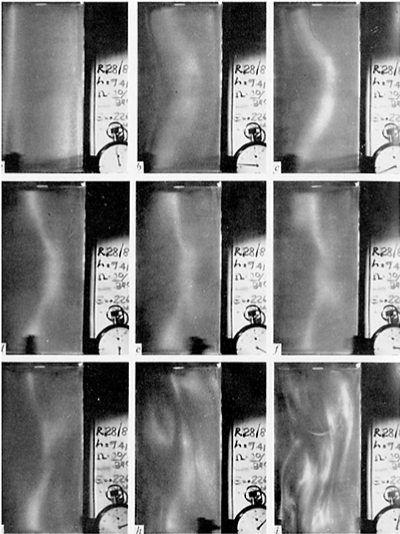
Figure 2 Time sequence demonstrating resonant collapse. (Reprinted with permission of the Cambridge University Press, from McEwan, A.D., "Inertial oscillations in a rotating fluid cylinder," J. Fluid Mech. 40 , 603–640 (1970).)
