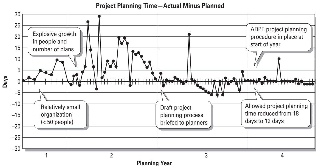
Figure 8–34 The figure shows a simple, yet insightful, way to show the effectiveness of part of an organization’s process—in this case, project planning. The plot, adapted from actual data, shows whether or not project plans were delivered late, on time, or early over a period of several years. Each point is a project plan ( x -axis) and its delivery date in days relative to its planned delivery date ( y -axis). If the y -value is positive, the plan was delivered late; if this value is zero, the plan was delivered on time; if this value is negative, the plan was delivered early.
