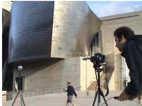
Figure 6.10. Capturing a Light Probe image in front of the museum with a mirrored ball and a digital camera.
