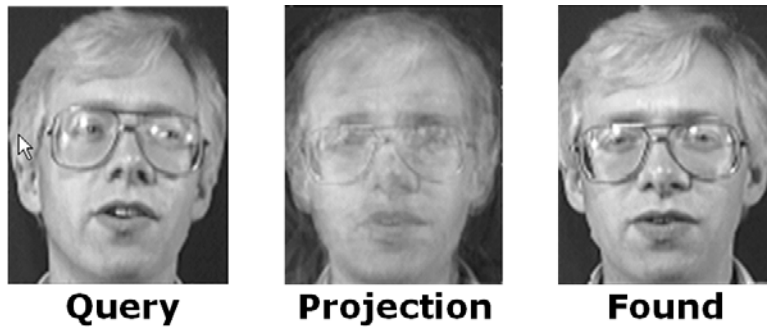
Figure 11.21. M5: Eigen face recognition example. Used with permission from [5, 6]
