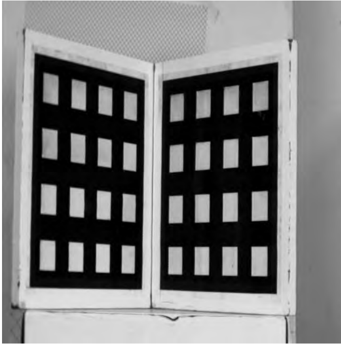
Figure 2.5. An example of camera calibration with a 3D apparatus
