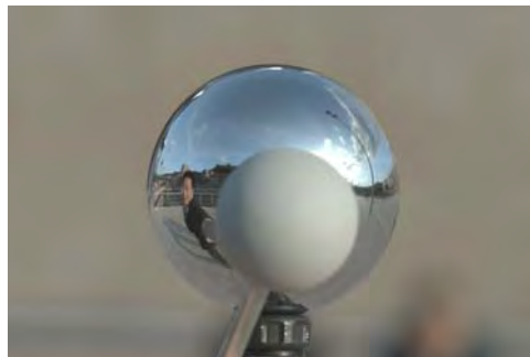
Figure 6.12. Photographing a diffuse grey sphere to determine the intensity of the sun.
