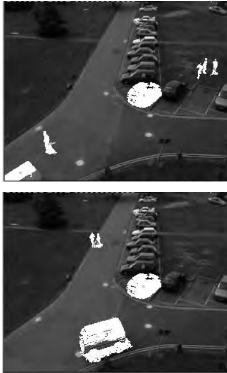
Figure 12.8. Object segmentation and tracking results in a PETS02 test sequence. The examples shown are two sample output composite frames taken at different times in the original video. The original colors have been altered to highlight the segmented blobs (in white) in the color to grey scale conversion required for printing.
