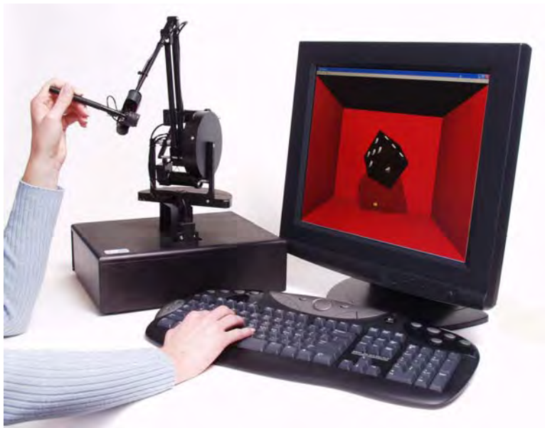
Figure 10.4. SensAble Technologies, Inc. PHANTOM haptic input/output device (reprinted with permission).
