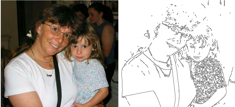
Figure 11.33. Interface Matlab: Left image is the input, right image is after running Canny on it with low/high thresholds 120/200. .
