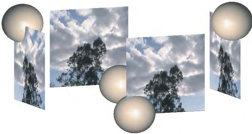
Figure 12.18. A rendered frame of the (animated) 3-D model with texture mapping from a live video stream.
