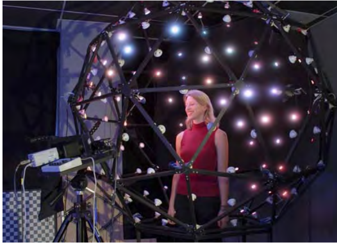
Figure 6.33. Light Stage 3. A subject is illuminated by a real-time reproduction of the light of Grace Cathedral.
