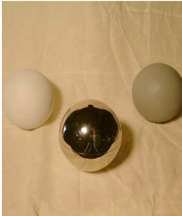
Figure 7.1. Chrome and diffuse balls used to capture environment maps.
