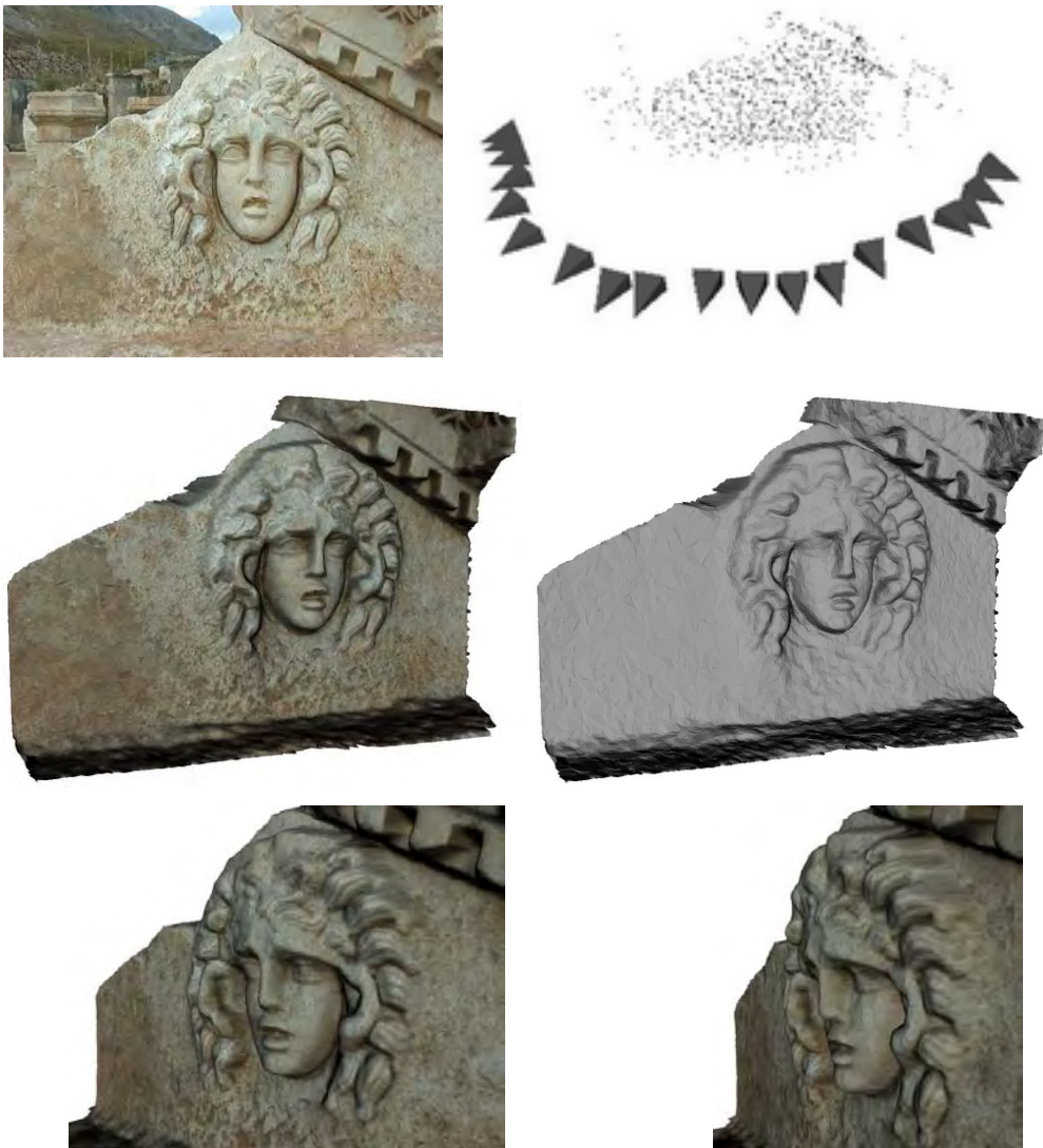
Figure 3.20. 3D-from-video: one of the video frames (upper-left), recovered structure and motion (upper-right), textured and shaded 3D model (middle) and more views of textured 3D model (bottom).
