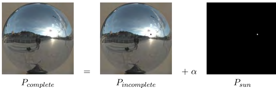
Figure 6.15. Modeling the complete image-based lighting environment the sum of the incomplete light probe image plus a scalar times a unit sun disk.
