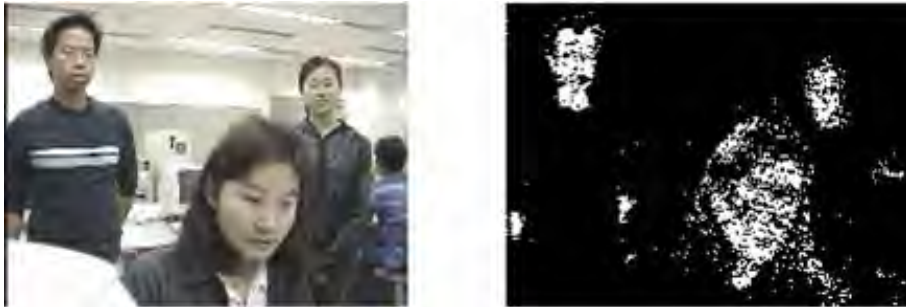
Figure 9.3. Skin color filtering: Input image with single (a) and multiple (c) people. Skin color filtered maps (b) and (d).
