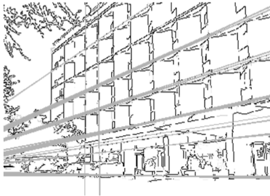
Figure 11.12. M2: Lines found by the Hough transform for lines. Used with permission from [5, 6]
