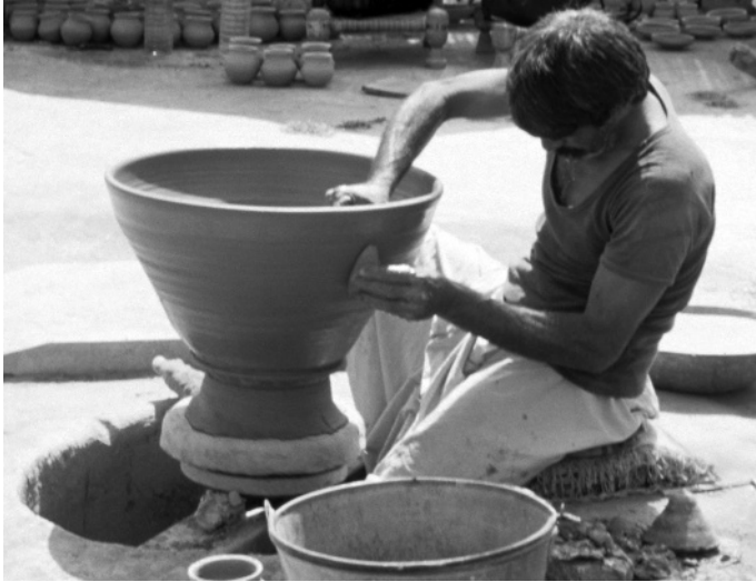
FIGURE 4.6 Zaman evening the base of a large vessel on a kick-wheel. The same kick-wheel is used as a tournette to add coils to the upper surface of large vessels whose bases are made in molds.
