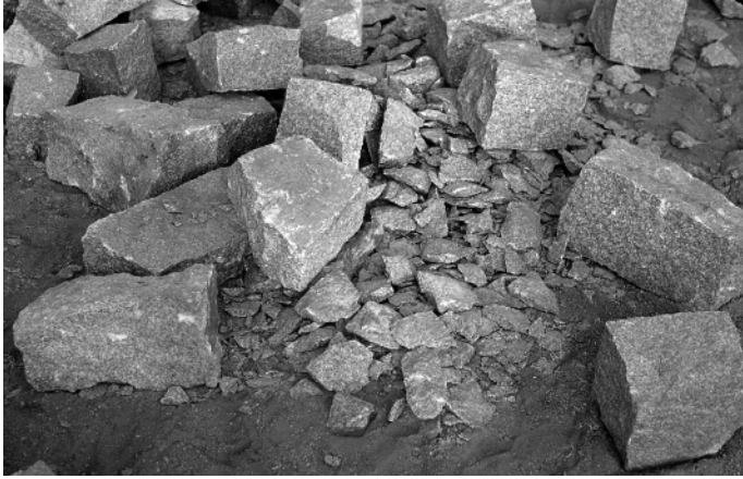
FIGURE 3.6 Creation of building stone blocks by knapping, using direct percussion with iron hammers.
