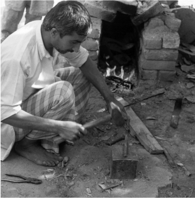
FIGURE 4.15 Blacksmith forging iron bar on expedient “anvil” in front of annealing fire.
