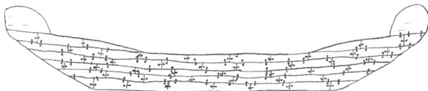
FIGURE 5.5 Sketch of Chumash tomal , a sewn wooden plank boat or “plank canoe.” (Redrawn after Arnold 2001.)
