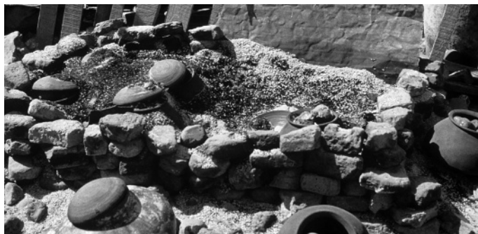
FIGURE 3.3 Heat treatment of agate nodules inside pottery vessels, using rice husks as fuel in a reducing atmosphere. Photo courtesy of Lisa Ferin.
