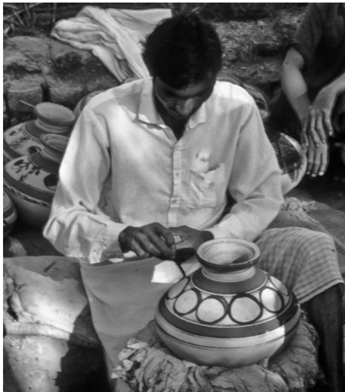
FIGURE 4.7 Nawaz painting the upper surface of a water jar on a kick-wheel used as a tournette.
