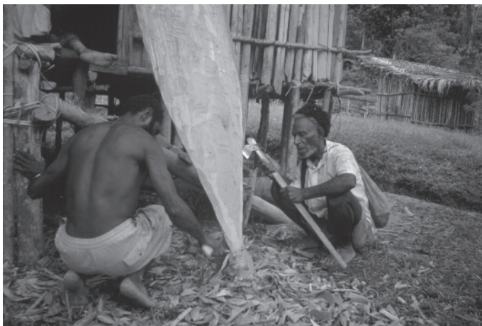
FIGURE 3.22 Bretaro shaping a wooden door board using an axe. Photo courtesy of Roger Ivar Lohmann.
