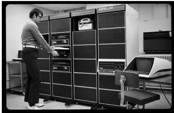
FIGURE 4-1 The first Regenstrief mainframe, a PDP-11/44. Doug Martin, an early system developer, is shown working with the system.
