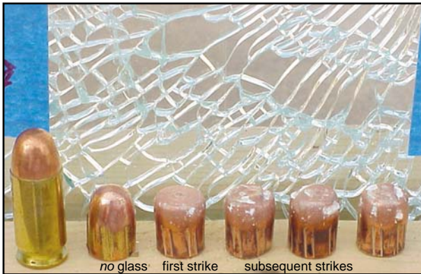
Color Plate 8 Shot Sequence and Facet Formation on Bullets through Tempered Glass (see Figure 6.18)
