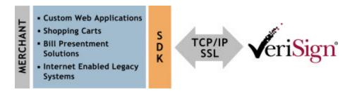
Payflow Pro SDK gives merchants more control via a direct TCP/IP connection to the payment gateway and a flexible Software Development Kit (SDK).
