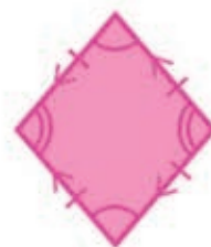
RHOMBUS This quadrilateral has four sides of equal length, and two pairs of opposite angles that are also equal.
