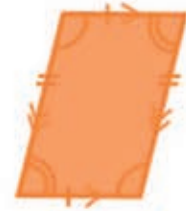
PARALLELOGRAM This has two pairs of equal-length sides and two pairs of equal angles. The opposite sides are parallel.
