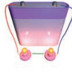
SERIES CONNECTION All the power moves through each part of the circuit, in a line.
