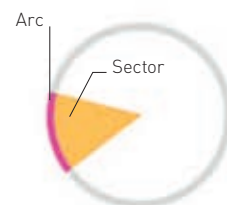
ARC AND SECTOR A sector is a space enclosed by two radii (the plural of radius). An arc is a section of the circumference.
