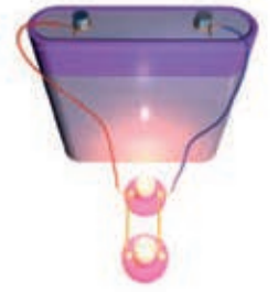
PARALLEL CONNECTION The power splits into two as it reaches two lamps wired like this.
