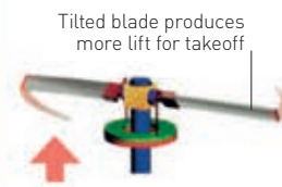
Flatter blade produces less lift while landing
