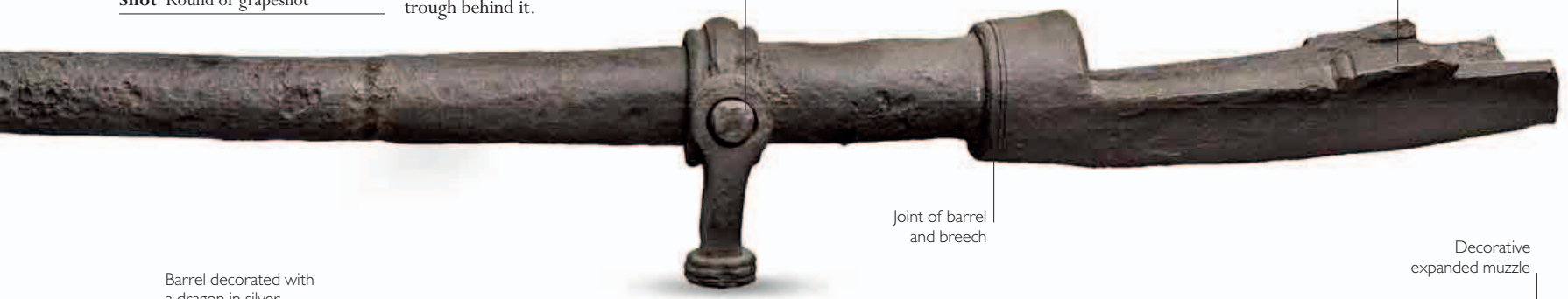
Trunnions, rounded projections on the sides of the barrel, help to elevate and lower muzzle
