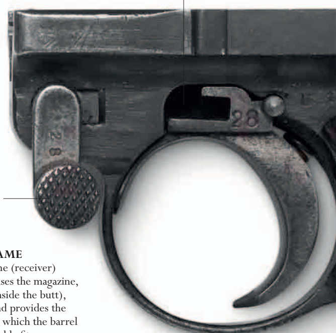
Slot in trigger mechanism for sear link lever
