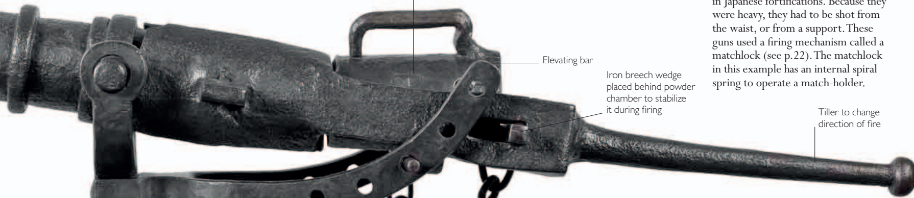
Tankard-shaped powder chamber
