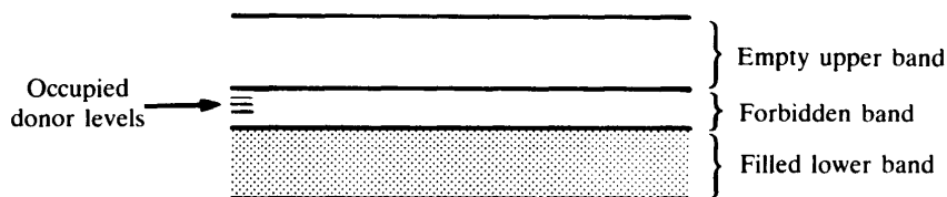
Fig. 35-7 Energy bands of an n -type semiconductor.
