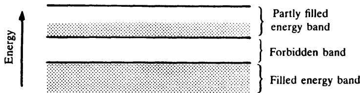
Fig. 35-3 Energy bands of a metal.
