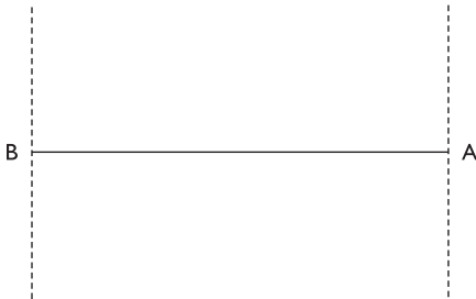
Figure 5.5 Suggested limits for the location of points by intersection.
