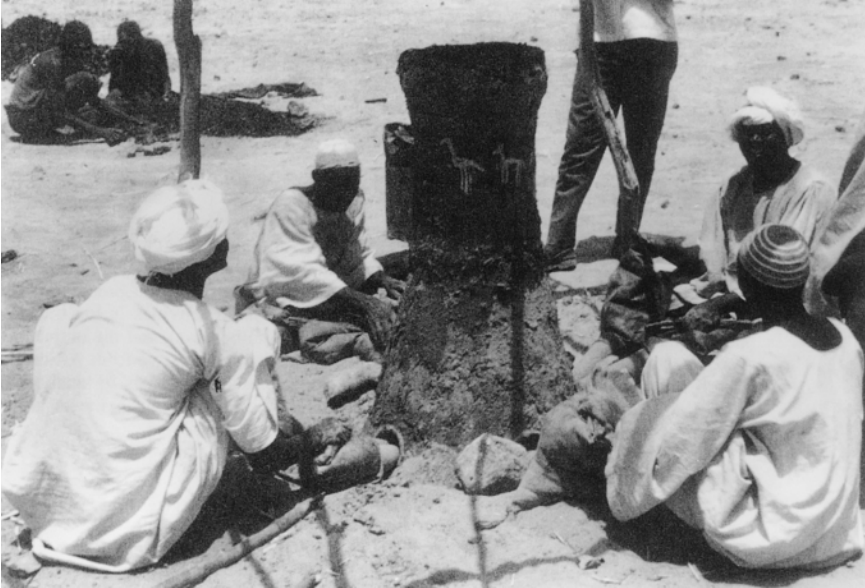
Figure 21 Bloomery furnace being prepared for smelting iron, Toumra, western Sudan. Reproduced by permission of Gunnar Haaland from Haaland, G. and others 2002. The social life of iron. Anthropos 97, Figure 2.
