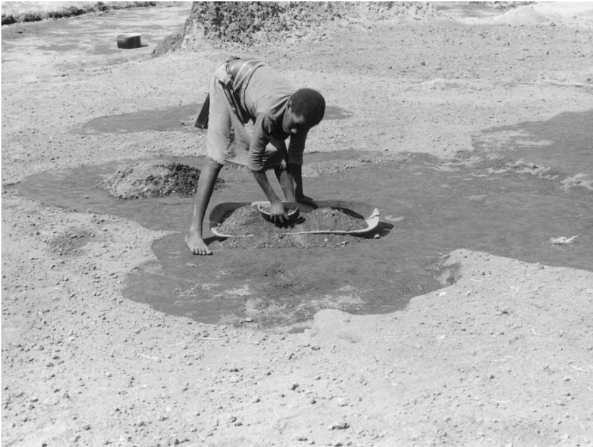
Figure 58 Salt production at Kibiro, Uganda. Earth, previously scattered on the ground to absorb salt, is scraped up prior to leaching and boiling the resulting brine.
