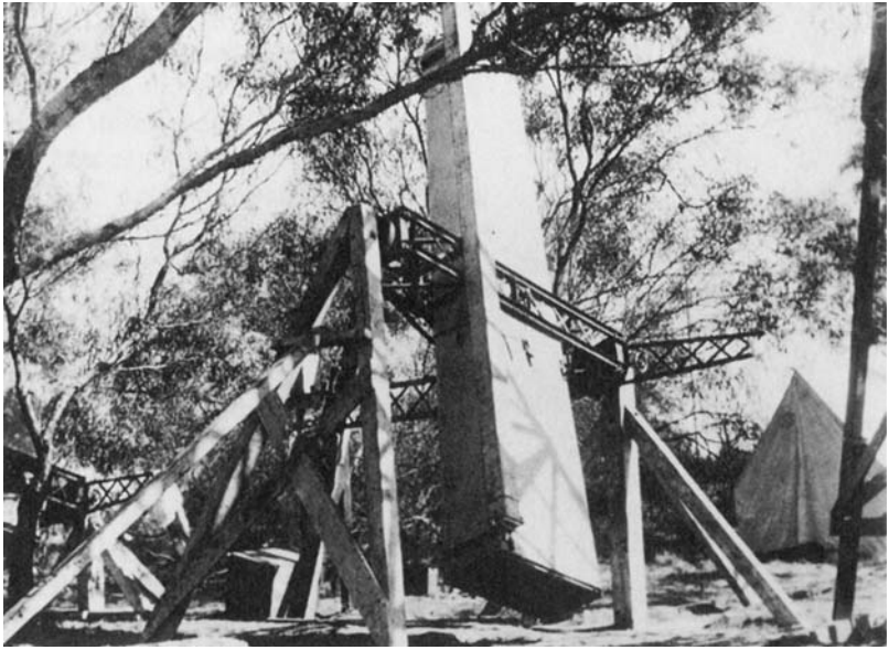
Makeshift mount for the principal telescope used by the Lick Observatory team to test relativity at the 1922 eclipse in Wallal, Australia. [Mary Lea Shane Archives of the Lick Observatory]
