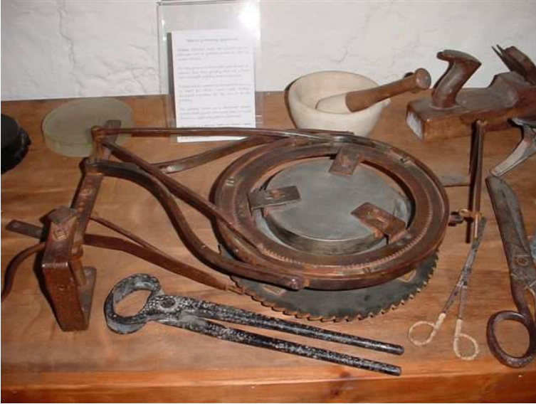
FIG. 4.5. A grinding-cum-polishing machine and other tools used by Herschel. The mirror being ground is the circular disc in the centre, which is face down above the tool. Between them would be the grinding paste: the mirror would become concave and the tool convex as the handle to the left was used to move the mirror back and forth over the tool. The ratchets would have given a small rotary action after each stroke. (Author's photograph, taken in the William Herschel Museum, Bath.)
