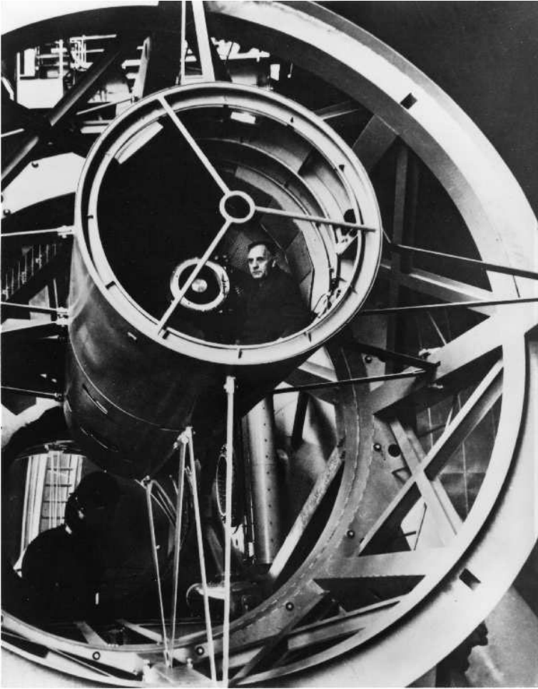
FIG. 9.8. Hubble posing in the 'prime focus cage' at the top of the 200-in. telescope. When used at prime focus, the telescope is at its most efficient. The light from a faint object is reflected only once, directly from the primary mirror, far below (Carnegie Institution of Washington).
