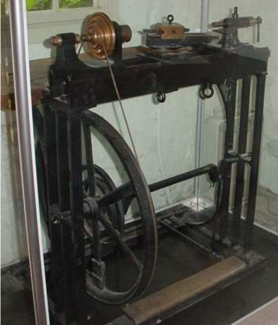
FIG. 4.1. Treadle lathe used by Herschel and his brother Alexander for making small telescope parts. The lathe is today in the William Herschel Museum in Bath (author's photograph).
