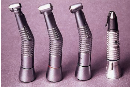
Fig. 5.12 A selection of low-speed handpieces. From the left: 1:1 ratio contra-angle handpiece used for most procedures. Latch-grip burs are used. Commonly identified with a blue-coloured band on the shank of the handpiece and a blue dot on the head. Speed in the range 400–40 000 rev/minute.
