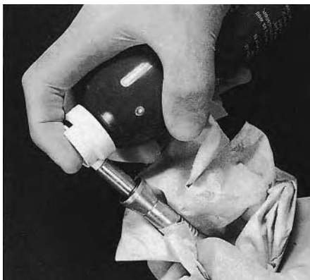
Fig. 5.13 An aerosol lubricant being used with a low-speed handpiece. Different adaptors for the nozzle of the aerosol are available for each type of handpiece. The paper towel is used to absorb excess lubricant coming through the head of the handpiece.
