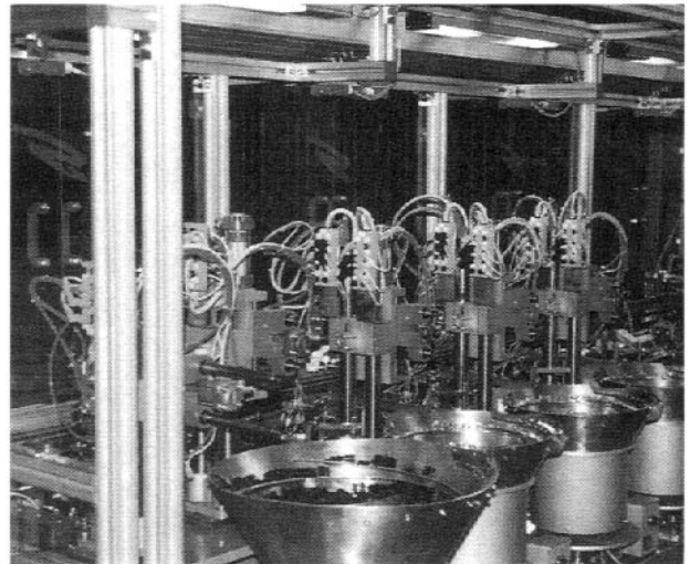
FIGURE 16-7. A Small Parts Fixed Automation Assembly Machine. In the foreground are parts feeders that operate by vibration. The parts crawl up the helical track and are picked up at the top. Also visible are several work heads that can make simple up-down or in-out motions. They are operated by air pressure controlled by valves operated by a central controller. (Photo courtesy of Assemblagio .)
