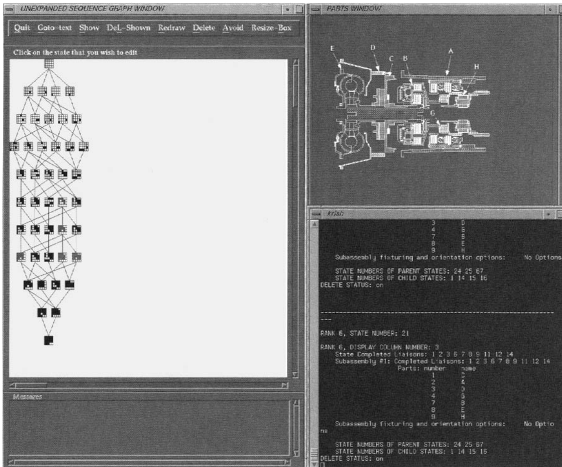
FIGURE 7-10. Sample Window from Draper/MIT Assembly Sequence Software. This window shows a phase of editing the sequences of a large truck automatic transmission. The state illustrated in the parts window at the upper right is the one that is in the 7th row, 4th position from the left, in the sequence diagram at the left. The lower right window allows commands to be typed in. A row of command buttons is available at the top left. These permit the user to delete states or transitions or to request that the diagram be redrawn.
