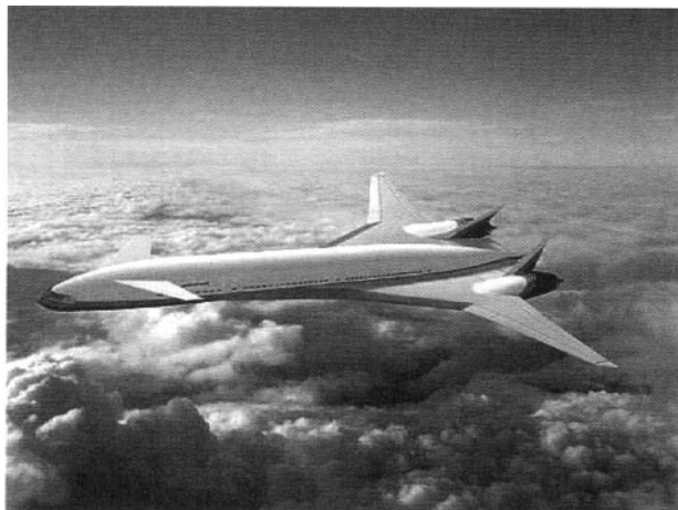
FIGURE 14-19. Artist's Rendition of Boeing Sonic Cruiser Concept. (Courtesy of Boeing. Used by permission.)
