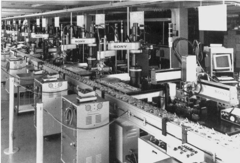
FIGURE 17-22. A Line of Sony Robots Assembling VCR Recording Heads. Twenty-five of these robots assembled a total of about hundred parts. Each robot was equipped with a turret of up to five tools, shown in Figure 17-23. (Photo courtesy of Sony FA.)
