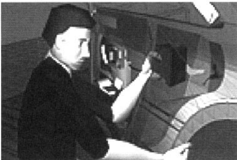
FIGURE 17-16. Human Simulation Software Jack Performing an Automotive Assembly Task. Jack is sold by EDS, a CAD and factory design company. (Image taken from http://www.plmsolutions-eds.com/products/efactory/jack/ . Used by permission.)
