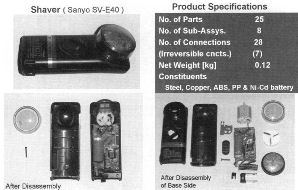
FIGURE 15-20. Shaver Used for DfDRR Example. ([Kanai, Sasaki, and Kishinami]. Courtesy of S. Kanai. Used by permission.)
