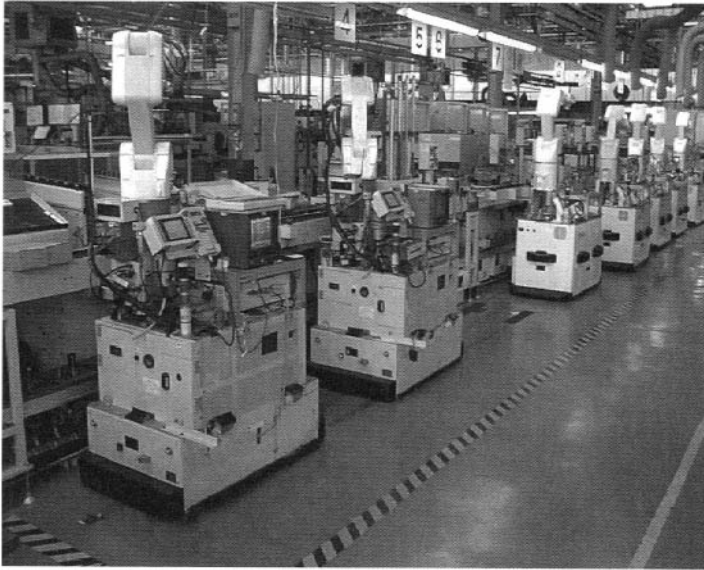
FIGURE 16-31. Denso Roving Robot Line for Starters. In this system, robots are not assigned to a specific assembly station but can cluster under decentralized control at places where excess work has accumulated. The line is similar to cells discussed in Section 16.F.6 in the sense that production rate can be varied by adding or removing robots from the line. The workpieces travel along a conveyor. Parts are fed from the side of the line opposite the robots. The robots carry a suite of tools and pick up the tool needed by the next part at whatever station they are attending. ([Hanai et al.]. Copyright © IEEE 2001. Used by permission.)
