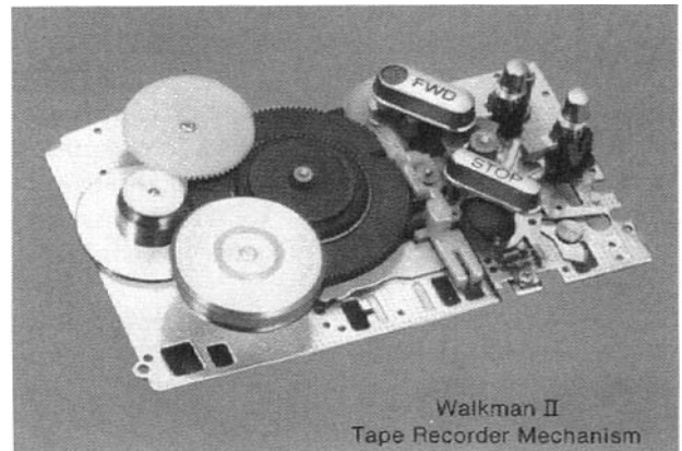
FIGURE 14-15. The Walkman II Recorder Chassis. In this version of the product, the circuit board is a separate unit. In later versions, after surface mount electronics were introduced, the mechanical chassis and the circuit board became the same unit. This process improvement permitted much thinner units to be made. (Photo courtesy of Sony FA.)
