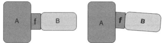
FIGURE 3-16. Two Parts Constrained by Joining Assembly Features. Left: The nominal situation. Right: The situation if the feature “f” on part A is misoriented.
