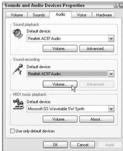
Figure 20-2: Set audio input and adjust the volume of input for a Windows PC.
