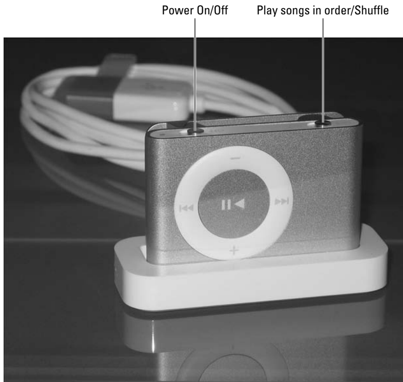
Figure 14-6: The iPod shuffle offers two switches: power on/off, and play songs in order/shuffle.
