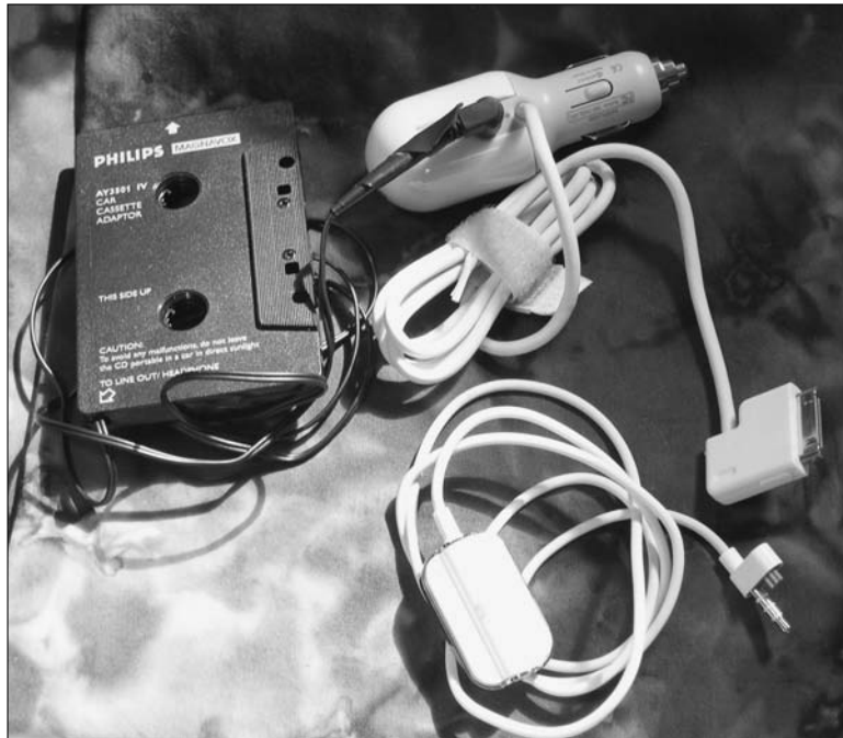
Figure 15-1: Inexpensive car accessories: cassette-player adapter (left); power adapter (upper right); and Apple Remote (lower right).
