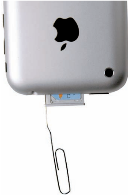
Figure 14-1: Removing the SIM tray.
