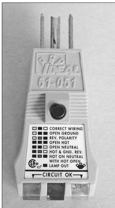
Figure 4-8: Receptacle and GFI tester close up.
