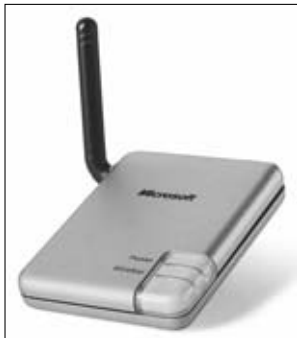
Figure 2-2: A wireless network adapter that attaches to a computer's USB port.
