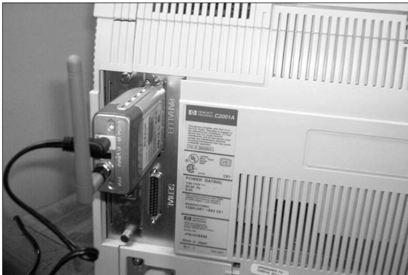
Figure 6-4: Wireless print server attached to a printer.
