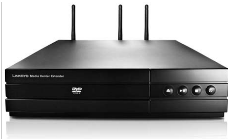
Figure 12-3: The DMA 2200 from Linksys will hook your Media Center PC to remote TVs.
