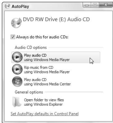
Figure 15-5: When you insert a CD, Windows Vista asks you what to do with it.
