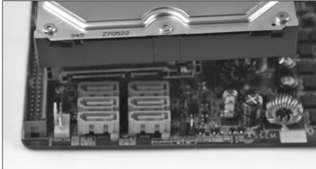
Figure 17-5: SATA drive positioned with left- facing SATA connector.
