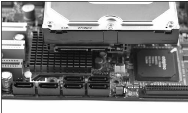
Figure 16-8: SATA drive controller connection.
