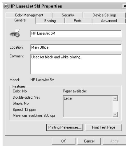
Figure 2-38: Use the General tab to find more about the printer and perform a basic test.
