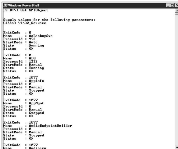
Figure 1-7: PowerShell usually tries to help you provide the minimum information necessary to use a Cmdlet.
