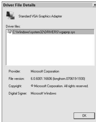
Figure 2-15: The list of driver files tells you the location of the driver on disk.
