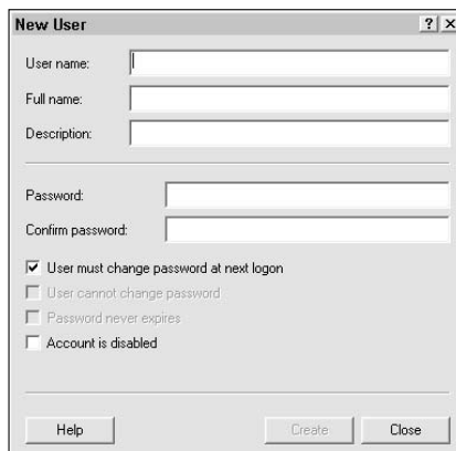
Figure 4-5: Use the New User dialog box to create new users for your server.
