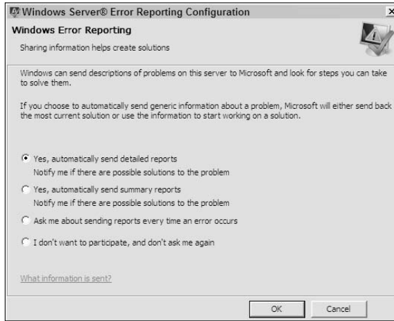
Figure 4-17: Let Windows do the work of checking for fixes to errors you encounter.
