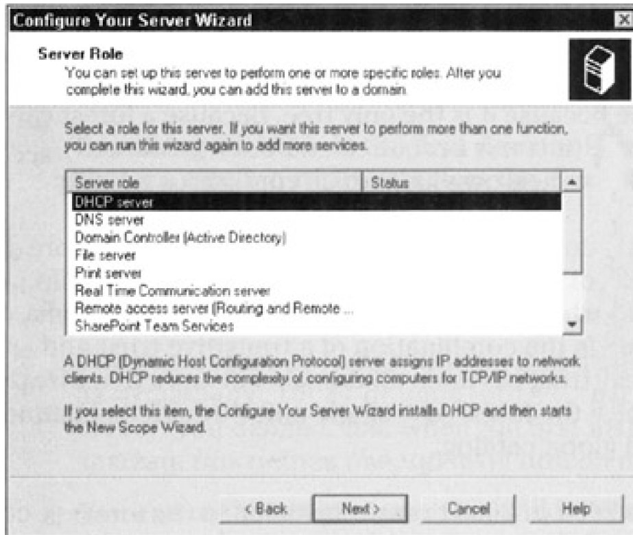
Figure 10-1: The server roles that can be installed through the Configure Your Server Wizard.
