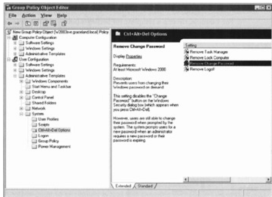
Figure 15-7: The Ctrl+Alt+Del options that can be set with the User Configuration Administrative Template.
