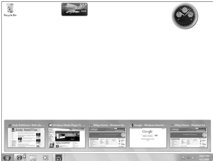
Figure 1-2: The new taskbar in Windows 7 offers pop-up thumbnail previews of every open window on your desktop.
