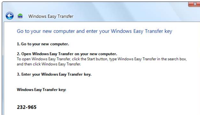
Figure 4-8: The Windows Easy Transfer key indicates that the From computer is ready to send data.
