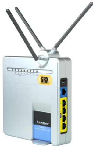
Figure 4-4: A wireless router has rabbit ears (in this case, three of them), slots for LAN cables, and a special slot for the Internet connection.
