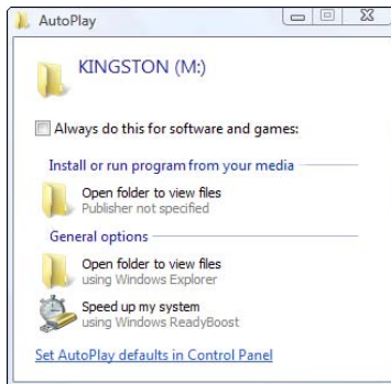
Figure 1-9: The entry marked Install or Run Program is bogus, generated by Conficker.
