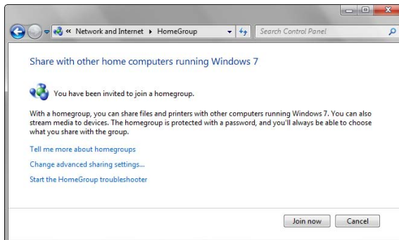
Figure 1-7: The invitation you receive the first time you connect to a network, if Windows finds a HomeGroup.
