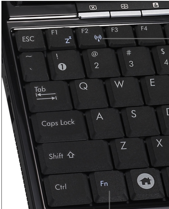
Figure 1-4: To enable (or disable) wireless on the Eee PC 1000H, hold down the Fn key and press F2.
