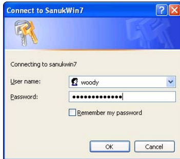
Figure 1-18: To get into a Windows 7 computer's \Public folder, provide a recognized username and password.
