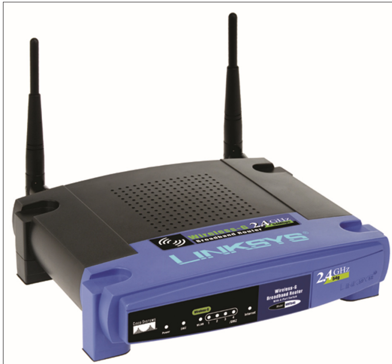
Figure 3-3: The Linksys WRT54G, a workhorse wireless access point and router.
