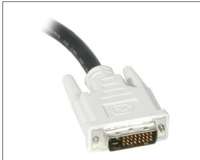
Figure 1-8: DVI-D has largely supplanted the old VGA video adapter.
