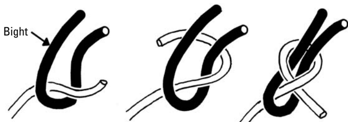
Figure 14-2: Tying a sheet bend.
