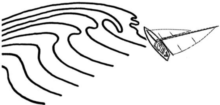
Figure 18-3: A plunging breaker.
