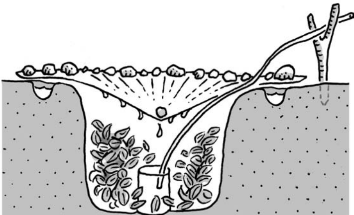
Figure 7-3: A basic solar still with vegetation.
