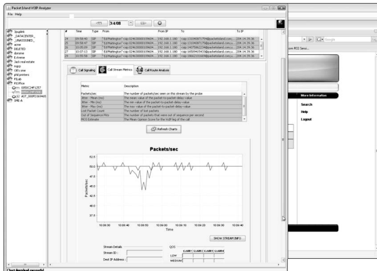
Figure 9-3: Packets per second call analysis detail.
